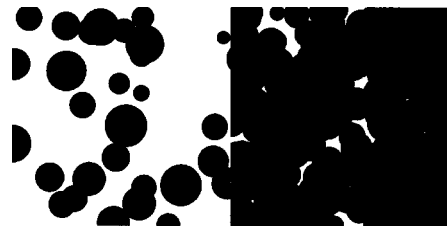
FIG. 1. Random disk Boolean model with log-normally distributed (dimensionless) radii, \beta = 0.25 and R_0 = 1 , with spatial intensity \rho = 0.1 on the left and \rho = 1.0 on the right.
