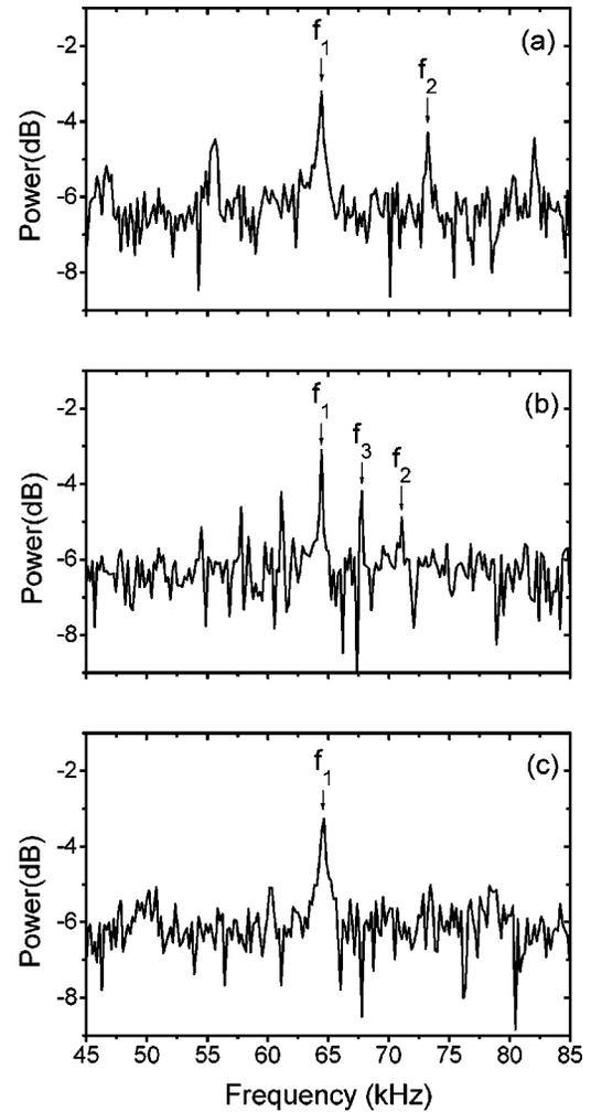
FIG. 4. Enlarged power spectra of Fig. 3. (a) Quasiperiodic state with  $f_1$  and  $f_2$ . (b) State of the period-doubled torus: quasiperiodic state with  $f_1$  and  $f_3 = f_1 + \Delta f/2$ . (c) Chaotic state.
