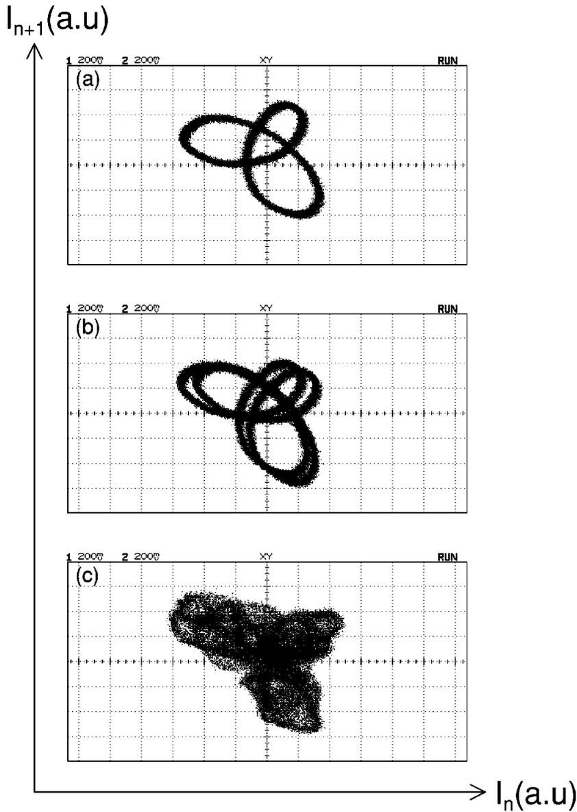
FIG. 6. Folded and separated case of torus doubling: (a) torus at  $f = 56.522$  kHz, (b) period-doubled torus at  $f = 56.538$  kHz, and (c) chaos at  $f = 56.547$  kHz.
