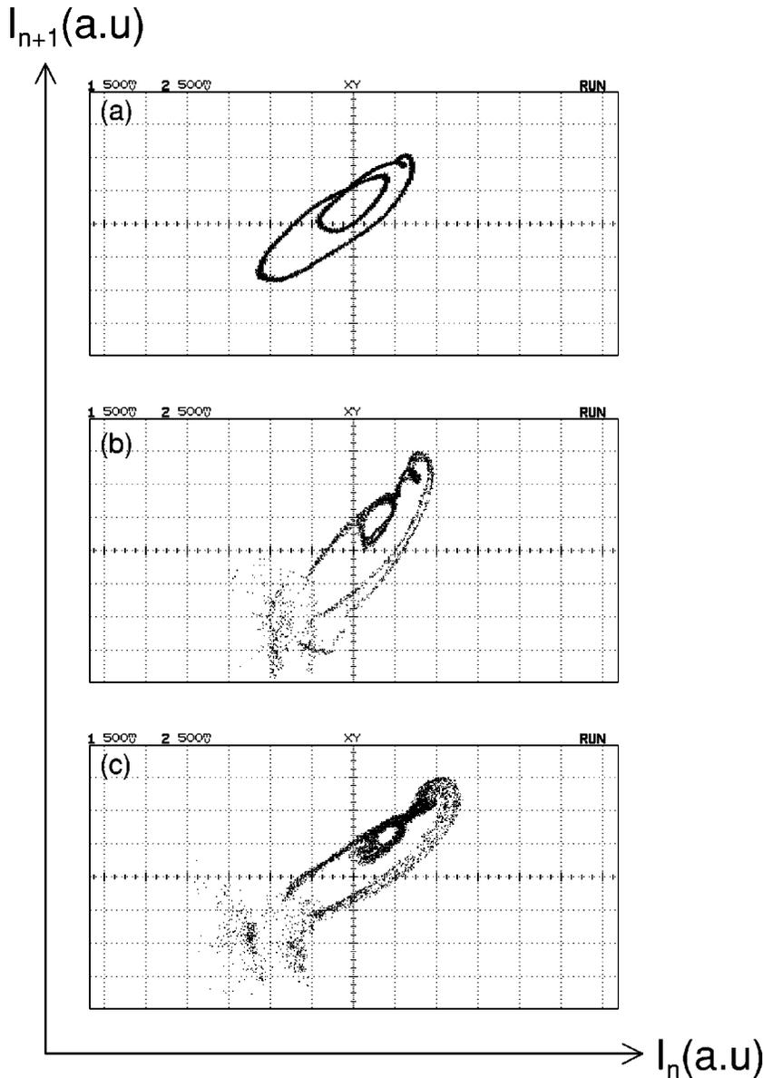
FIG. 1.  $I_{n+1}$  vs  $I_n$ .  $I_n$  is a local maximum of the current oscillation across the resistor. (a) Torus generated by the Hopf bifurcation at  $f=64.395$  kHz. (b) Period-doubled torus at  $f=64.431$  kHz. (c) Chaos at  $f=64.453$  kHz.
