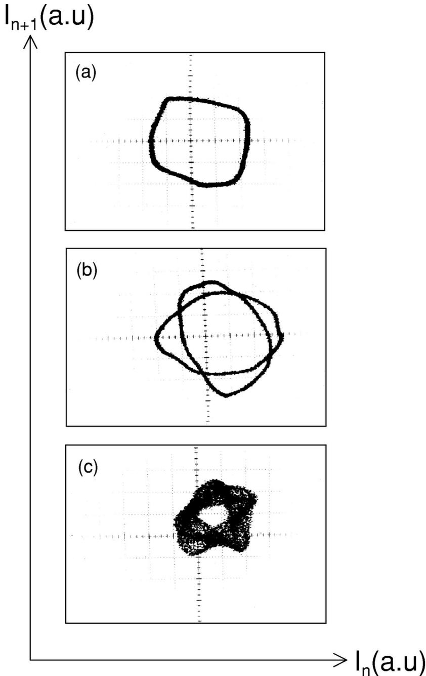
FIG. 5. Separated case of torus doubling: (a) torus at  $f = 62.092$  kHz, (b) period-doubled torus at  $f = 61.074$  kHz, and (c) chaos at  $f = 60.404$  kHz.
