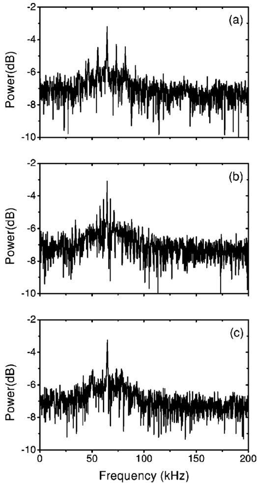
FIG. 3. Corresponding power spectra of the time series in Fig. 2. (a) Quasiperiodic state of two-incommensurate frequencies with  $f_1$  and  $f_2$ . (b) State of the period-doubled torus: quasiperiodic state with  $f_1$  and  $f_3 = f_1 + \Delta f/2$ . (c) Chaotic state.
