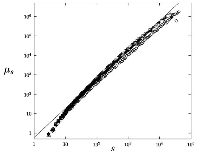
FIG. 2. First moment  $\mu_s$  vs the size  $s$  in log-log scale. The slope gives  $3 - \phi$ . The marks  $\diamond, +, \square, \times, \triangle, *$  correspond to 2,3,4,5,6,7 dimensions. The straight line is drawn with a slope 1.5 for eye guidance.
