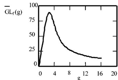
FIG. 2. Graph of the  $\overline{GL}_f(g)$  function in the case when the total electron number of the bunch,  $N^{(e)}$ , is an invariant value during the compression.
