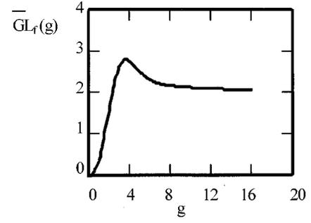
FIG. 1. Gain dependence on the length of an electron bunch in the natural logarithm scale. It is assumed that the bunch average density  $\rho_0$  is an invariant value; the bunch length is normalized by the wavelength of the amplified signal  $g = 2\pi l/\lambda$ .
