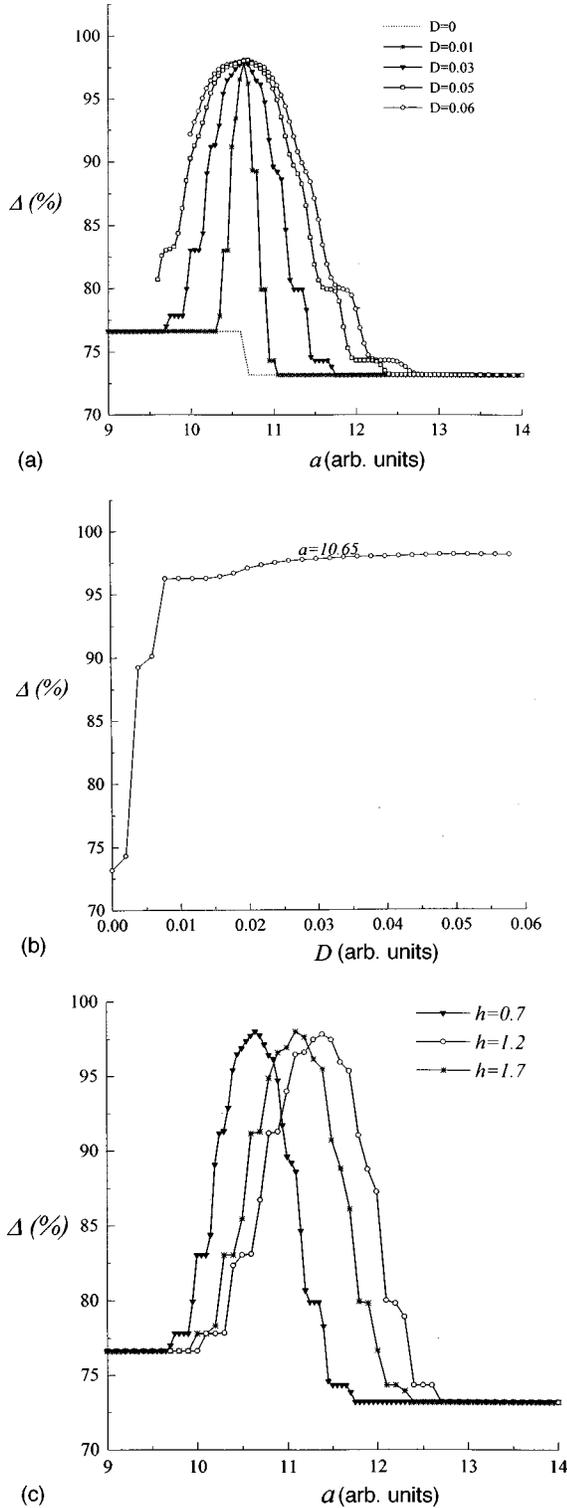
FIG. 4. Quality function  $\Delta$  [%] for pattern replication in a two-layer system. (a) Dependence of  $\Delta$  on the excitability parameter  $a$  for  $h=0.7$ . Different curves correspond to different fixed values of the intralattice diffusion  $D$ . (b) Evolution of the peak value of  $\Delta$  at  $a=10.65$  with increasing  $D$ . (c) Shift of the ‘‘resonance’’ quality with the parameter  $h$ . Units are arbitrary.
