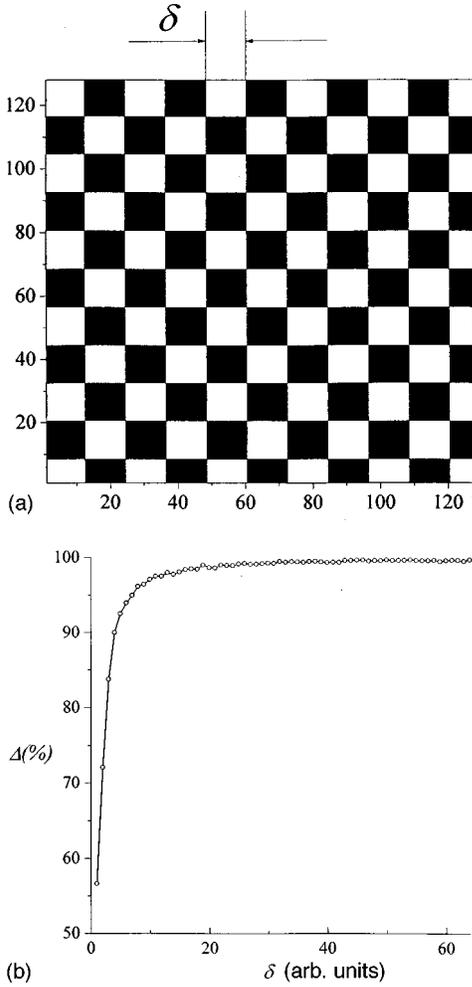
FIG. 8. (a) Pattern used to test the spatial resolution of the image replication system. (b) Dependence of the replication quality on the relative characteristic spatial scale of the test image  $\delta$ ,  $a = 10.6$ ,  $D = 0.06$ ,  $h = 0.7$ . Units are arbitrary.
