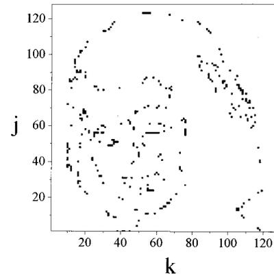
FIG. 3. Differential image obtained as the misprint signal between replicated copies [Fig. 2(c) and 2(d)] and the original image [Fig. 2(a)].
