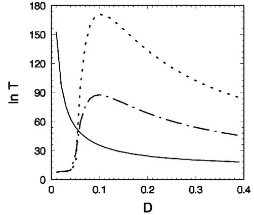
FIG. 4. The MFPT of the bistable system (12) as a function of  $D$  for  $\lambda=1$  and  $\alpha=0.05$  with  $\tau=0.1$  (straight line),  $\tau=0.02$  (dash-dotted line),  $\tau=0.01$  (dotted line).
