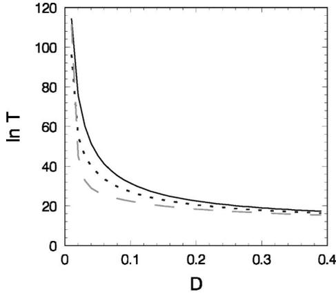
FIG. 3. The MFPT of the bistable system (12) as a function of  $D$  for  $\lambda=1$  and  $\tau=0.1$  with  $\alpha=0.1$  (straight line)  $\alpha=0.18$  (dotted line),  $\alpha=0.3$  (dashed line).
