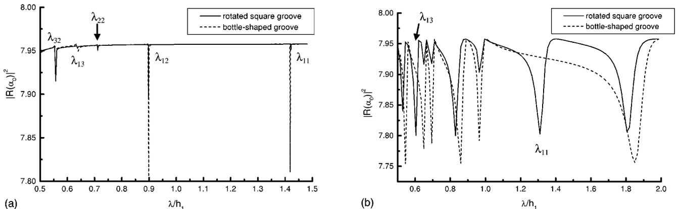
FIG. 8. Comparison between the intensity versus wavelength curves for a bottle-shaped ( $c_1=h_1$ ,  $c_2=0.1h_1$ , and  $h_2=0.01h_1$ ; dashed curve) and a rotated square groove ( $a=h_1$  and  $b=0.1h_1$ ; solid curve). The normally incident Gaussian beam has width  $w=100h_1$ . (a)  $s$  polarization and (b)  $p$  polarization.
