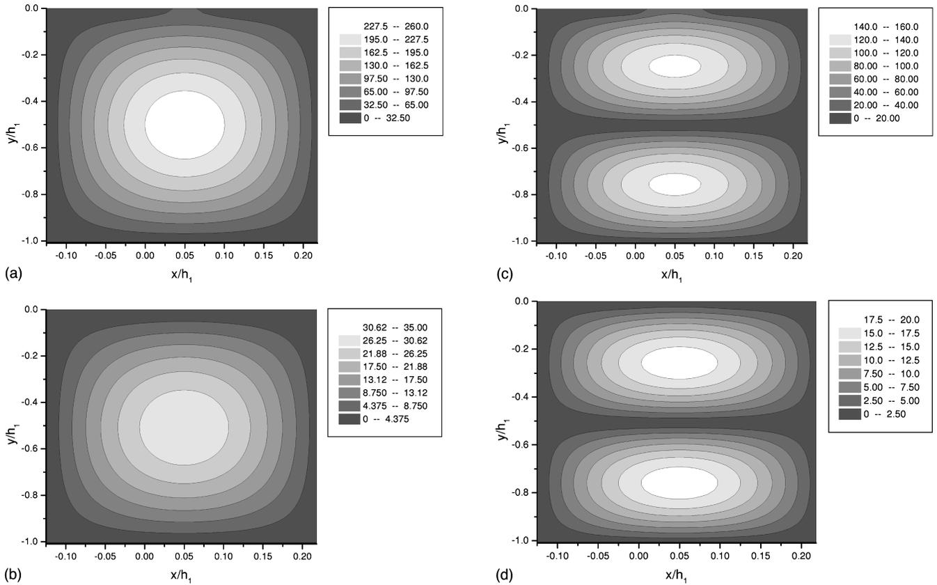
FIG. 6. Absolute value of the electric field inside a bottle-shaped groove of the same parameters considered in Fig. 5,  $c_2=0.1h_1$  and for  $s$  polarization, for four values of the incident wavelength: (a)  $\lambda=0.662h_1$ , (b)  $\lambda=0.661h_1$ , (c)  $\lambda=0.5765h_1$ , and (d)  $\lambda=0.5741h_1$ .
