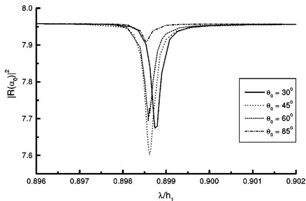
FIG. 9. Intensity reflected in the specular direction versus wavelength, for a bottle-shaped groove with the same parameters considered in Fig. 8 and  $s$  polarization, for  $\theta_0 = 30^\circ$ ,  $45^\circ$ ,  $60^\circ$ , and  $85^\circ$ .
