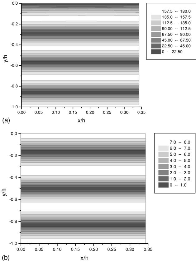
FIG. 4. Absolute value of the magnetic field inside a rectangular groove of the same parameters considered in Fig. 2 and for  $p$  polarization, for different incident wavelengths: (a)  $\lambda = 0.57h$  and (b)  $\lambda = 0.66h$ .
