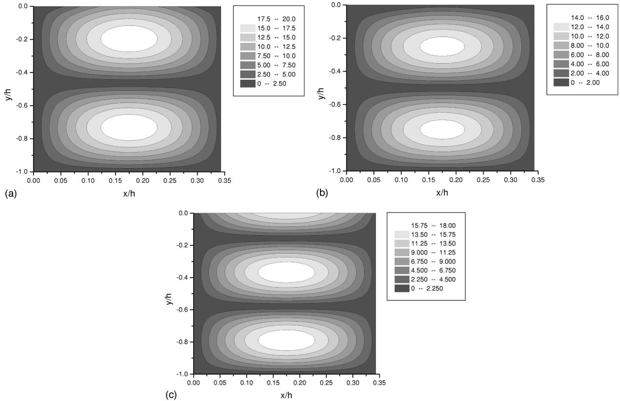
FIG. 3. Absolute value of the electric field inside a rectangular groove of the same parameters considered in Fig. 2 and for  $s$  polarization, for different incident wavelengths: (a)  $\lambda = 0.586h$ , (b)  $\lambda = 0.5734h$ , and (c)  $\lambda = 0.5386h$ .
