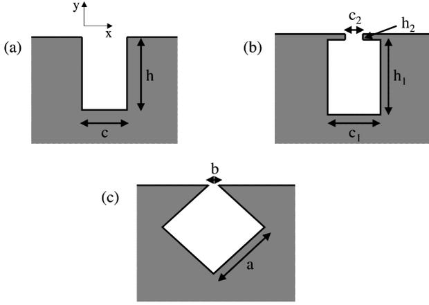
FIG. 1. Rectangular profiles of the cavities considered: (a) open rectangular, (b) bottle shaped, and (c) bivalued.
