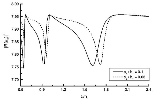
FIG. 7. Intensity reflected in the normal direction versus wavelength, for a bottle-shaped groove of  $c_1=0.35h_1$ ,  $h_2=0.01h_1$ , and for different values of  $c_2$ :  $0.1h_1$  and  $0.03h_1$ . The normally incident Gaussian beam is  $p$  polarized and has width  $w=100h_1$ .
