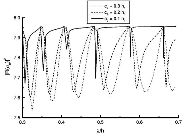
FIG. 5. Intensity reflected in the normal direction versus wavelength, for a bottle-shaped groove of  $c_1 = 0.35h_1$ ,  $h_2 = 0.01h_1$ , and for different values of  $c_2$ :  $0.3h_1$ ,  $0.2h_1$ , and  $0.1h_1$ . The normally incident Gaussian beam is  $s$  polarized and has width  $w = 100h_1$ .
