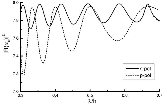
FIG. 2. Intensity reflected in the normal direction versus wavelength, for an open rectangular groove of width-to-depth ratio  $c/h = 0.35$ . The normally incident Gaussian beam has width  $w = 100h$ . The solid curve corresponds to  $s$  polarization and the dashed one corresponds to  $p$  polarization.
