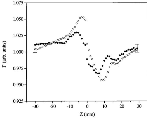
FIG. 3. Typical Z-scan result (normalized transmittance  $\Gamma$  as a function of the position  $z$ , 35 ms pulse; 185 mW power) with sample  $M_1$  at the  $N_c$  phase. Electric field of the polarized laser beam perpendicular to  $\mathbf{n}$ : (●) undoped sample; (○) ferrofluid-doped (3  $\mu\text{l/ml}$ ) sample. Typical error bars are shown.
