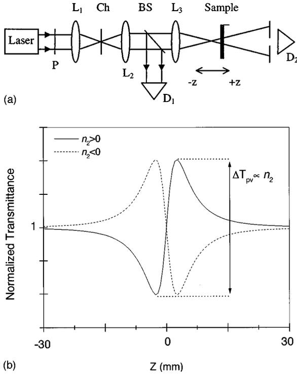
FIG. 1. (a) Sketch of the Z-scan apparatus.  $P$ , polarizer;  $Ch$ , chopper;  $L_1$ ,  $L_2$ , and  $L_3$ , lens;  $BS$ , beam sampler;  $D_1$  and  $D_2$ , detectors. (b) Theoretical behavior of the normalized transmittance as a function of the  $z$  position for two signs of the nonlinear refractive index  $n_2$ . The peak-to-valley distance  $\Delta T_{pv}$  is proportional to  $n_2$ .
