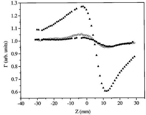
FIG. 2. Z-scan curves (normalized transmittance  $\Gamma$  as a function of the position  $z$ ; 35 ms pulse, 185 mW power) of the lyotropic mixture  $M_2$  at the isotropic phase, with different ferrofluid concentrations: (●) undoped sample; (○) ferrofluid-doped (3  $\mu l/ml$ ) sample; (▲) ferrofluid-doped (9  $\mu l/ml$ ) sample.
