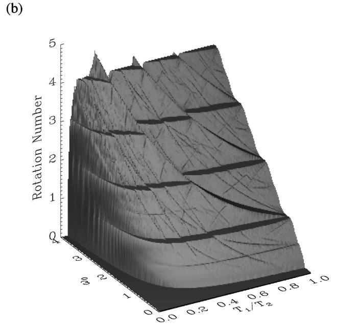
FIG. 4. Quasiperiodically forced circle map: (a) Three-frequency devil's staircase for forcing frequencies  $f_1 = 1, f_2 = 12/7$ . (b) Devil's ramps: the rotation number as a function of the external frequency ratio and the intrinsic frequency shows the global organization of three-frequency resonances.
