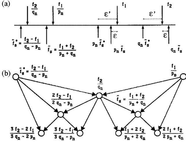
FIG. 1. (a) Schematic diagram of the frequency line, showing the relative position of  $\tilde{f}_s$  and  $\tilde{f}_s^*$  and their respective  $p_n, q_n$  harmonics that approximate  $f_1$  and  $f_2$  at equal distance. (b) Generalized Farey tree starting from the adjacent  $f_1/p_n$  and  $\tilde{f}_s^*$ . The first median is  $f_2/q_n$ ; at the second level we obtain  $\tilde{f}_s$  and  $(2f_2 - f_1)/(2q_n - p_n)$ , and so on.
