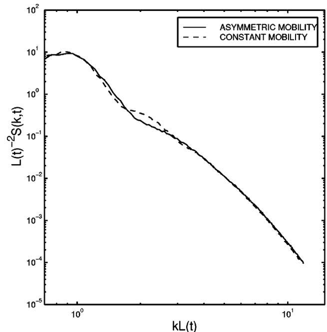
FIG. 6. Log-log plot of  $L^{-2}(t)S(k,t)$  vs  $kL(t)$  at time  $t=3000$  for the asymmetric mobility case and the constant mobility case with  $M(\phi)=1$ .
