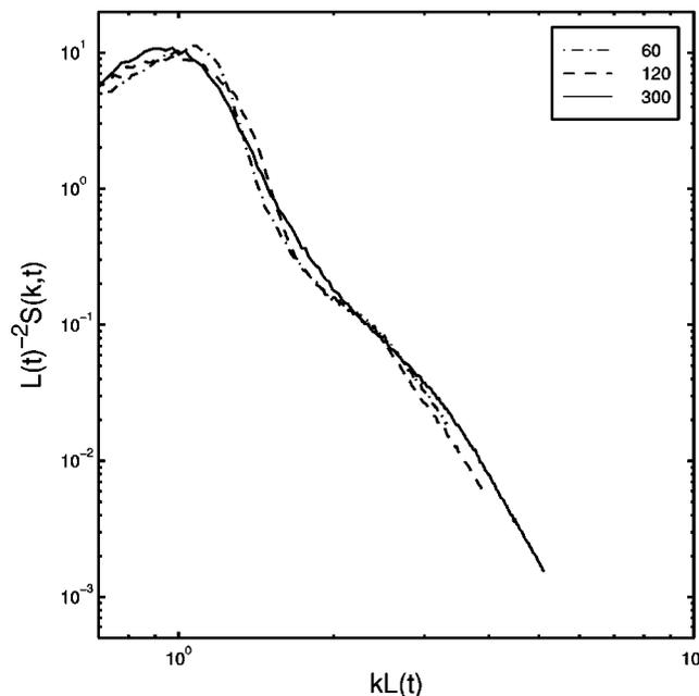
FIG. 4. Test for dynamical scaling in the early stages. We plot  $L^{-2}(t)S(k,t)$  vs  $kL(t)$  on a log-log scale for times  $t=60, 120,$  and  $300$ .
