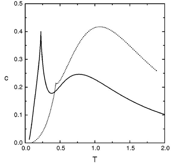
FIG. 1. Specific heat for the simple diamond lattice ( $p=q=2$ ) for the coupling constants  $J_A=0.1$ ,  $J_B=1$  (solid curve) and  $J_A=1$ ,  $J_B=0.1$  (small dashed). The critical exponent  $\alpha$  remains invariant.
