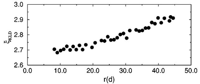
FIG. 3. Radial inhomogeneities of the length  $\xi_{\text{KLD}}$  in annular subsystems of fixed radii and increasing azimuthal angle for the  $\Gamma=109$  convection cell ( $\epsilon=0.79$ ). The radial distance  $r$  is measured in units of  $d$  (the thickness of the convection cell) from the center of the  $\Gamma=109$  convection cell.
