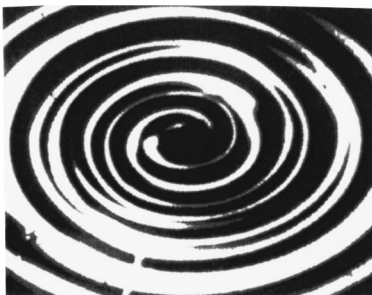
FIG. 3. Picture from above of the surface waves generated by the rotating bump (spiral waves).
