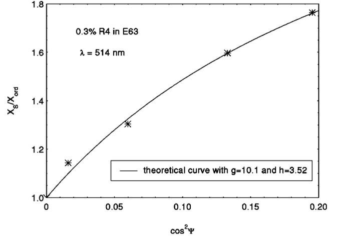
FIG. 2. Comparison of the theoretical curve [Eq. (7)] with the experimental points. To calculate the  $\Psi$  angle, the refractive indices of *E63* were used,  $n_o = 1.52$  and  $n_e = 1.75$ .
