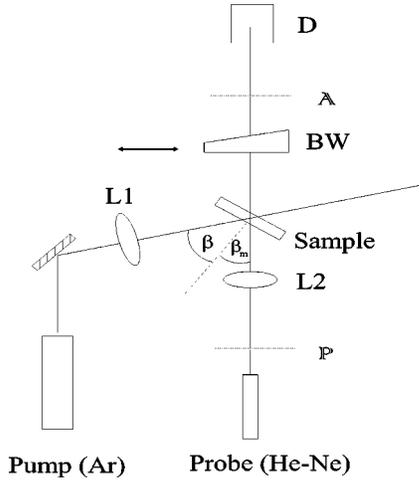
FIG. 3. Experimental setup used to measure the enhancement factor.  $P$ : polarizer;  $A$ : analyzer;  $BW$ : birefringent wedge;  $D$ : detector. The focal length of the  $L1$  and  $L2$  lens was 27 and 10 cm, respectively.
