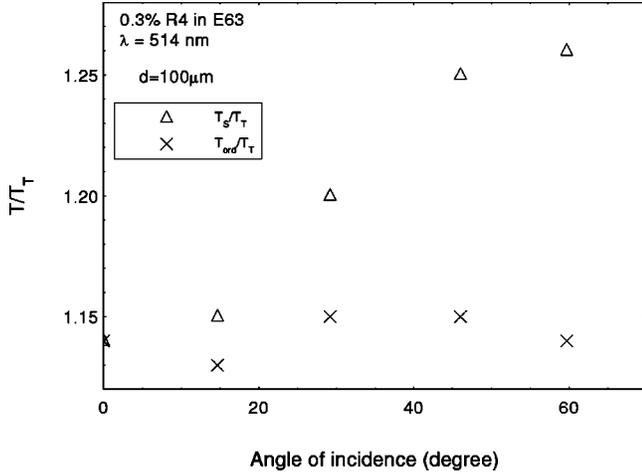
FIG. 1. Transmission of the probe beam, normalized to the initial transmission,  $T_T$ , at different angles of incidence of the pump beam. Pump power 6 mW, spot radius 1 mm. Angle of incidence of the probe beam  $45^\circ$ .
