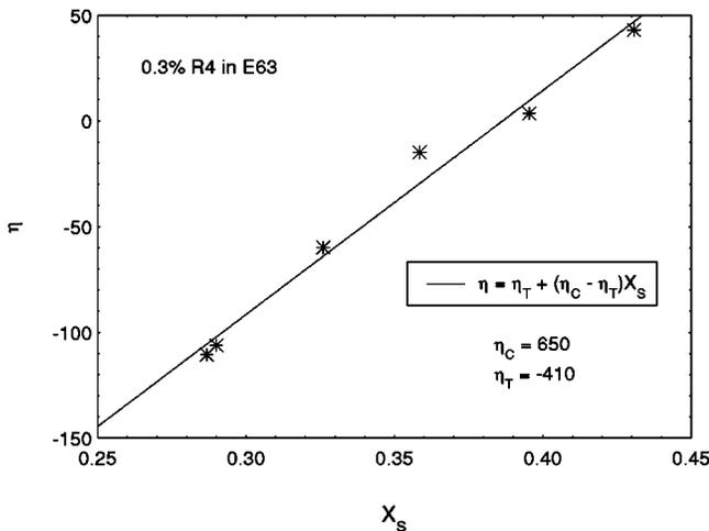
FIG. 6.  $\eta$  as a function of the *cis* fraction,  $X_S$ .  $X_S$  was calculated using Eq. (7) with  $X_{\text{ord}} = 0.26$ ,  $g = 10.1$ , and  $h = 3.52$ .
