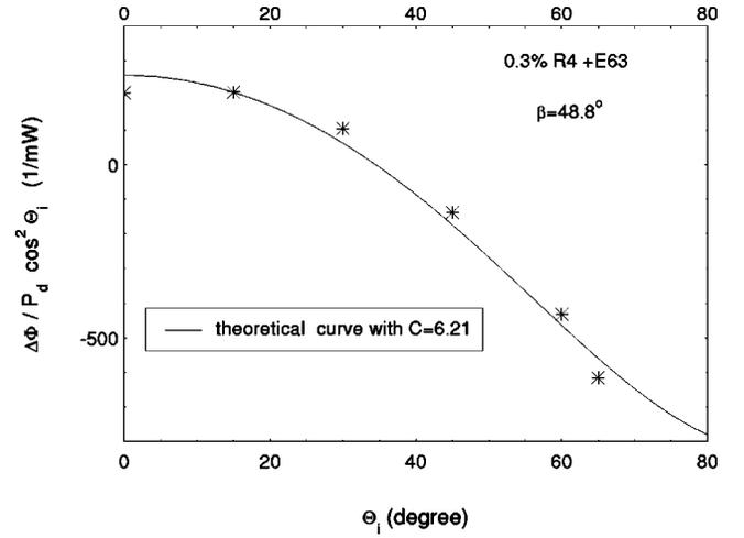
FIG. 7. Normalized phase shift as a function of the polarization angle of the input beam. Input powers were in the range 0.1–0.2 mW. The fitted curve corresponds to Eq. (26).
