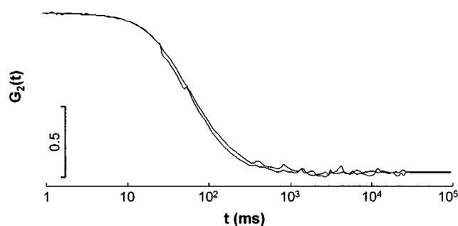
FIG. 3. ACFs of  $\beta$ -carotene particles (particle diameter 220 nm, measured at  $1510\text{ cm}^{-1}$ ), pure (lower curve, 1 wt %  $\beta$ -carotene in suspension) and in the presence of polystyrene lattices (upper curve, latex particle diameter 49 nm, particle number ratio latex/ $\beta$ -carotene 90, 0.5 wt %  $\beta$ -carotene in suspension). The ACF of the sample with the lattices has been scaled by a factor 0.61 to match the height of the ACF of the pure sample [16].
