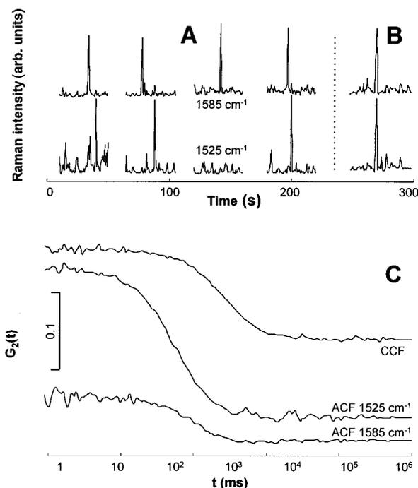
FIG. 4. Dual channel experiments with mixtures of  $\beta$ -carotene and vitamin A acetate. Channel 1 is set to  $1525\text{ cm}^{-1}$ , channel 2 to  $1585\text{ cm}^{-1}$ . (a) Intensity traces (channel 1 lower, channel 2 upper curves) showing the channels fluctuating independently. (b) Intensity trace showing a simultaneous signal in both channels. (c) Autocorrelation and cross-correlation functions from the mixture [16].
