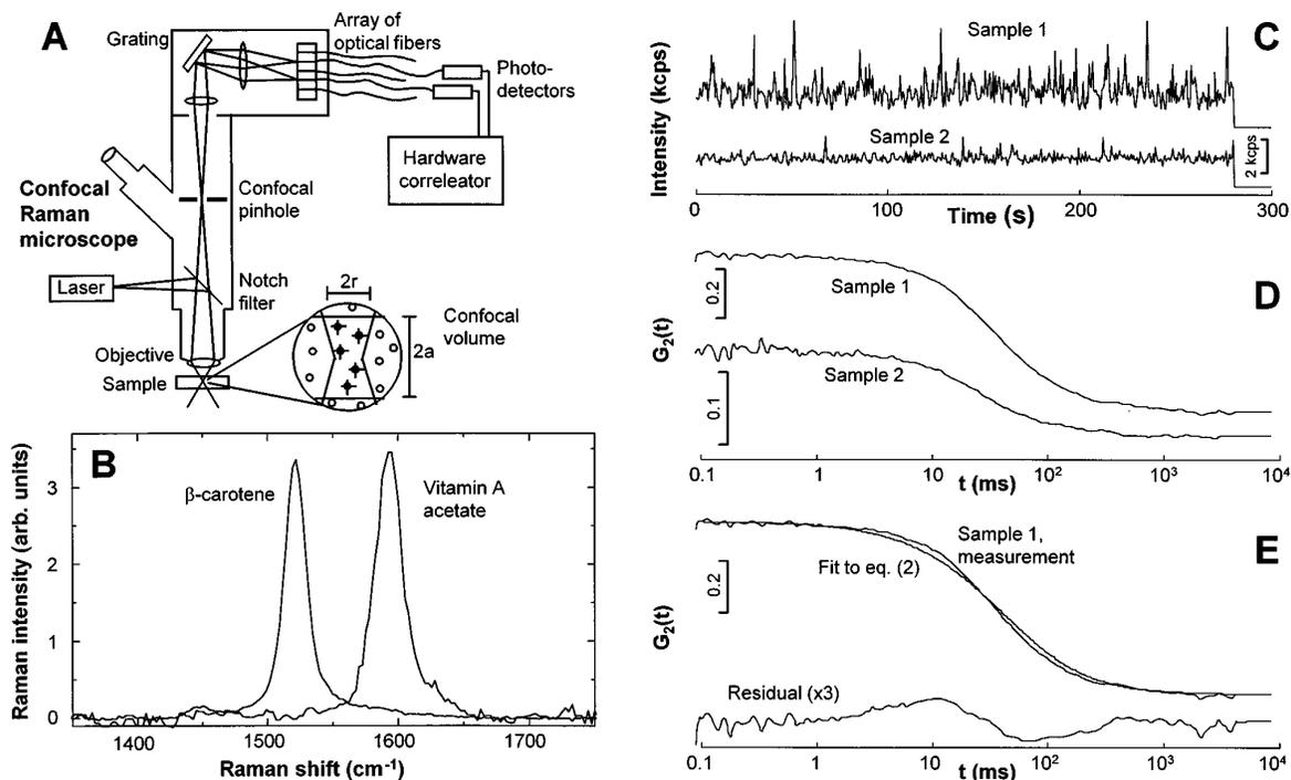
FIG. 1. Overview of the RCS technique. (a) Instrumental setup. (b) Raman spectra of the carotenoids of this study. (c) Raman intensity traces at  $1510\text{ cm}^{-1}$  from two different  $\beta$ -carotene dispersions. Sample 1: particle diameter 220 nm; sample 2: 150 nm, 1 wt %  $\beta$ -carotene in suspension. (d) ACFs resulting from the intensity traces. (e) Comparison of a fit of Eq. (2) to the ACF of sample 1, the residual has been magnified  $3 \times$  [16].
