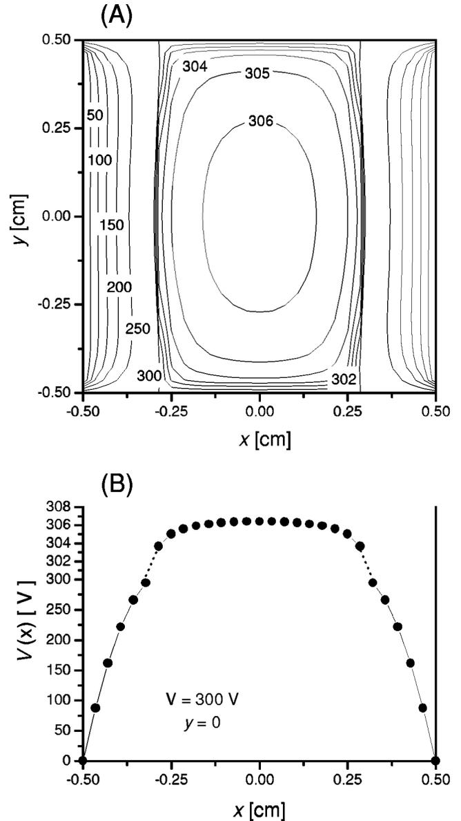
FIG. 3. (a) Potential distribution in the cross section of the rectangular hollow cathode discharge for  $p=2$  mbar and  $V=300$  V. (Data are given in volts.) (b) Potential distribution along the X axis. (Note that the scale is changed above 300 V.)
