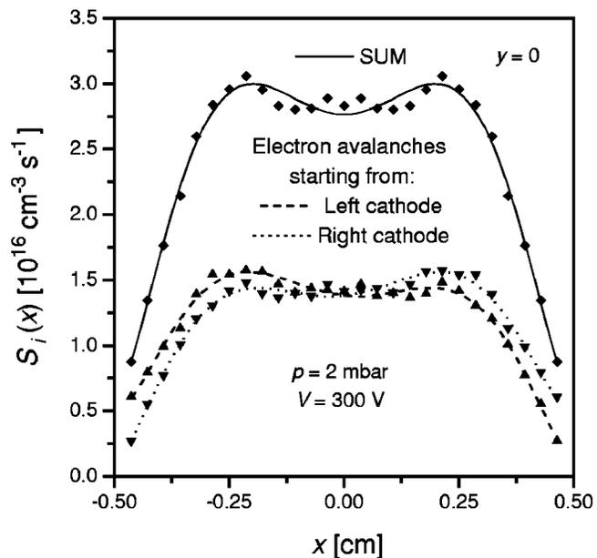
FIG. 9. Ionization source function  $S_i(x)$  (on the X axis) plotted by the solid line is the sum of source functions corresponding to electron avalanches starting from the “left” and “right” cathodes.
