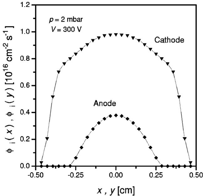
FIG. 4. Flux of  $\text{He}^+$  ions to the cathodes [ $\phi_i(y)$ ] and to the anodes [ $\phi_i(x)$ ] for  $p=2$  mbar and  $V=300$  V.
