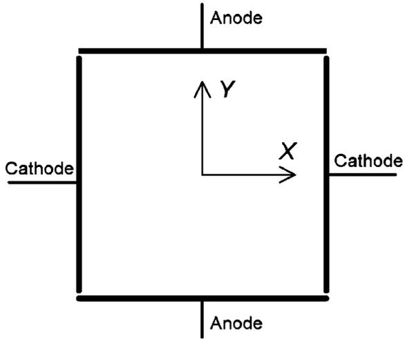
FIG. 1. Cross section of the rectangular hollow cathode discharge, indicating the Cartesian coordinate system used in the calculations. Electrodes of same polarity are separated by  $D=1$  cm. The discharge is infinite in the  $z$  direction [perpendicular to the  $(X,Y)$  plane].
