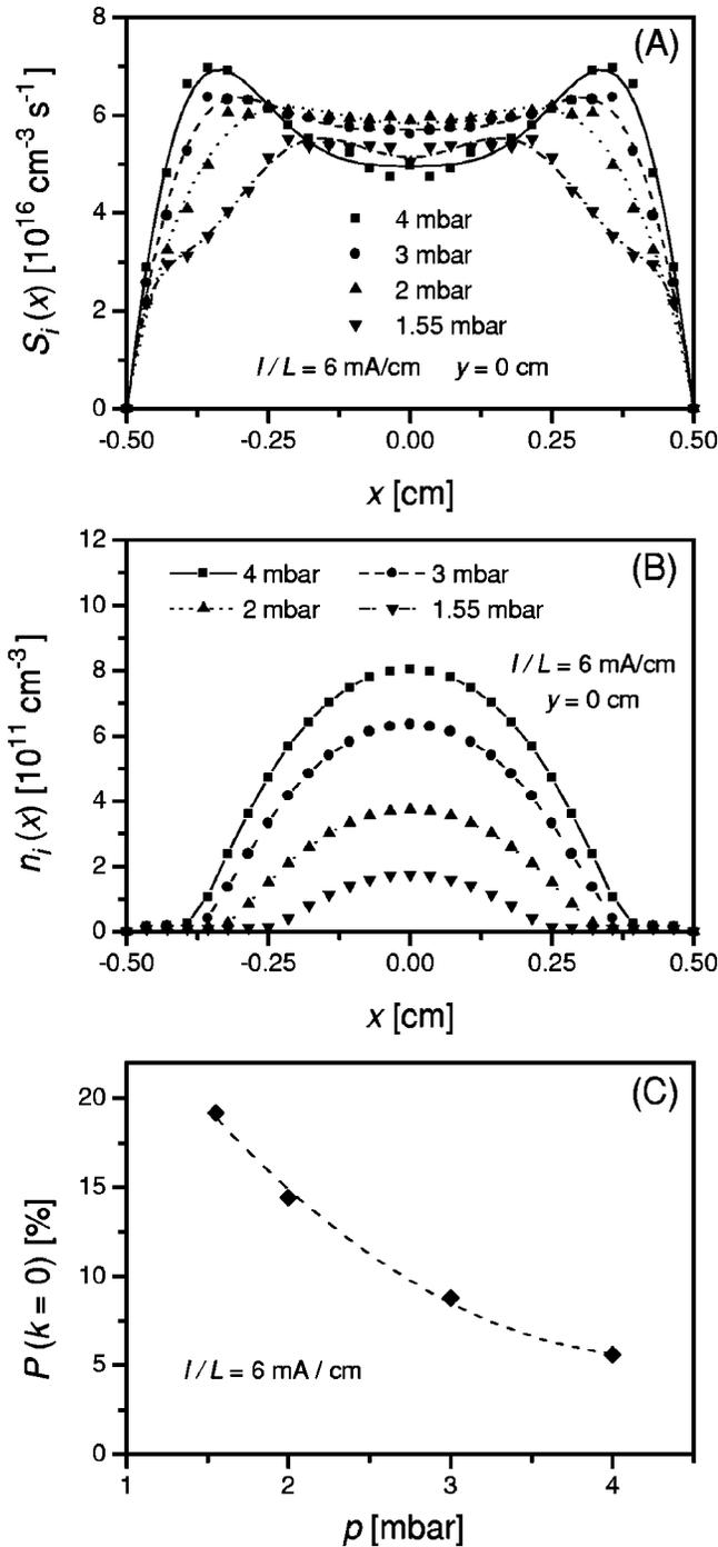
FIG. 11. Ionization source function  $S_i(x)$  (a), He $^+$  density  $n_i(x)$  (b) and the probability of producing zero ions in electron avalanches (c) for different values of helium pressure, at constant linear current density of  $I/L=6$  mA/cm.
