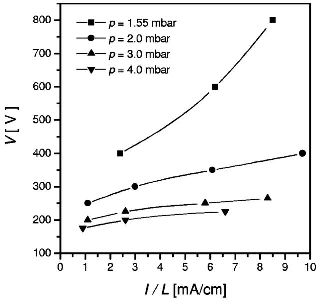
FIG. 2. Discharge voltage as a function of linear current density for different gas pressures.
