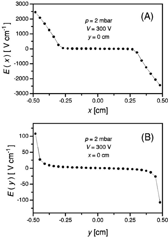
FIG. 6. Electric field distribution along the X axis (a) and the Y axis (b) of the discharge, for  $p=2$  mbar and  $V=300$  V.
