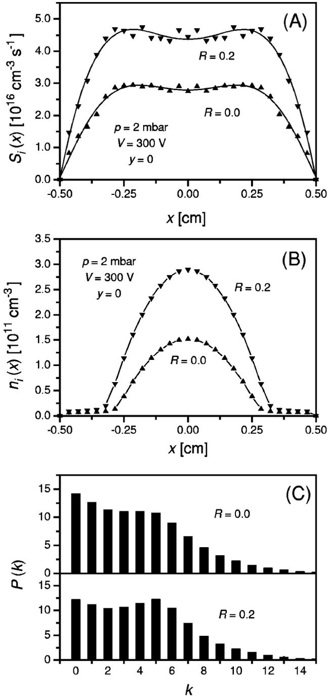
FIG. 12. Effect of backscattering of fast electrons from the anodes on the ionization source function  $S_i(x)$  (a) and  $\text{He}^+$  density  $n_i(x)$  (b). The  $P(k)$  distributions obtained at  $R=0.2$  and  $R=0.0$  (c) ( $p=2 \text{ mbar}$ ,  $V=300 \text{ V}$ ).
