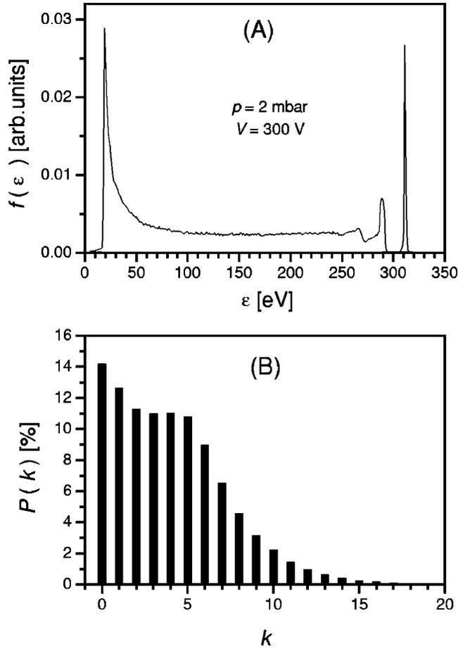
FIG. 8. (a) Energy distribution of fast ( $\epsilon > \epsilon_i = 24.6$  eV) electrons absorbed by the anode. (b) Statistical distribution of the number of ions created in electron avalanches ( $p=2$  mbar and  $V=300$  V).
