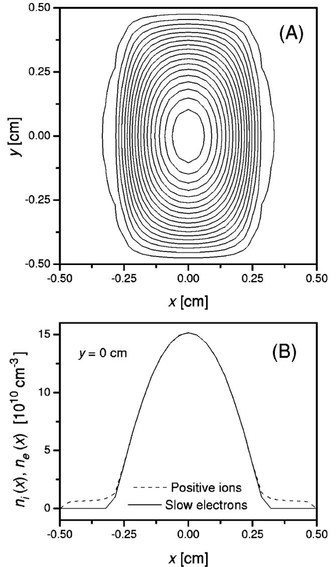
FIG. 5. (a) Two-dimensional density distribution of  $\text{He}^+$  ions. The distance of contour lines corresponds to  $10^{10} \text{ cm}^{-3}$  change of  $n_i(x,y)$ . (b) Density of  $\text{He}^+$  ions and slow electrons along the  $X$  axis ( $p=2$  mbar,  $V=300$  V)
