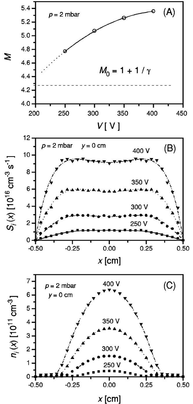
FIG. 10. Multiplication  $M$  of electrons (a), ionization source function  $S_i(x)$  (b) and  $\text{He}^+$  density  $n_i(x)$  (c) for different values of the discharge voltage, at constant pressure of  $p=2$  mbar.
