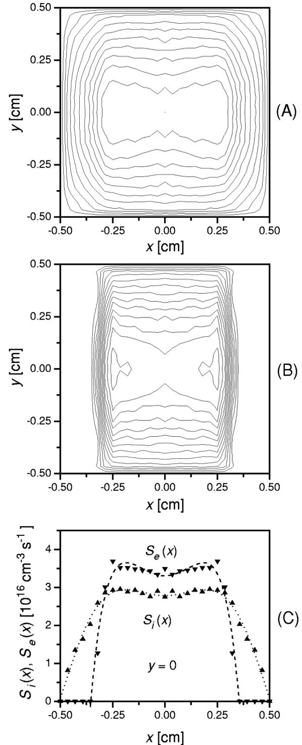
FIG. 7. Source function of  $\text{He}^+$  ions (a) and slow electrons (b) for  $p=2$  mbar and  $V=300$  V. The distance of contour lines corresponds to  $2.5 \times 10^{15} \text{ cm}^{-3} \text{ s}^{-1}$  change of the  $S_i(x,y)$  and  $S_e(x,y)$  source functions. (c) The  $S_i(x)$  and  $S_e(x)$  source functions on the X axis.
