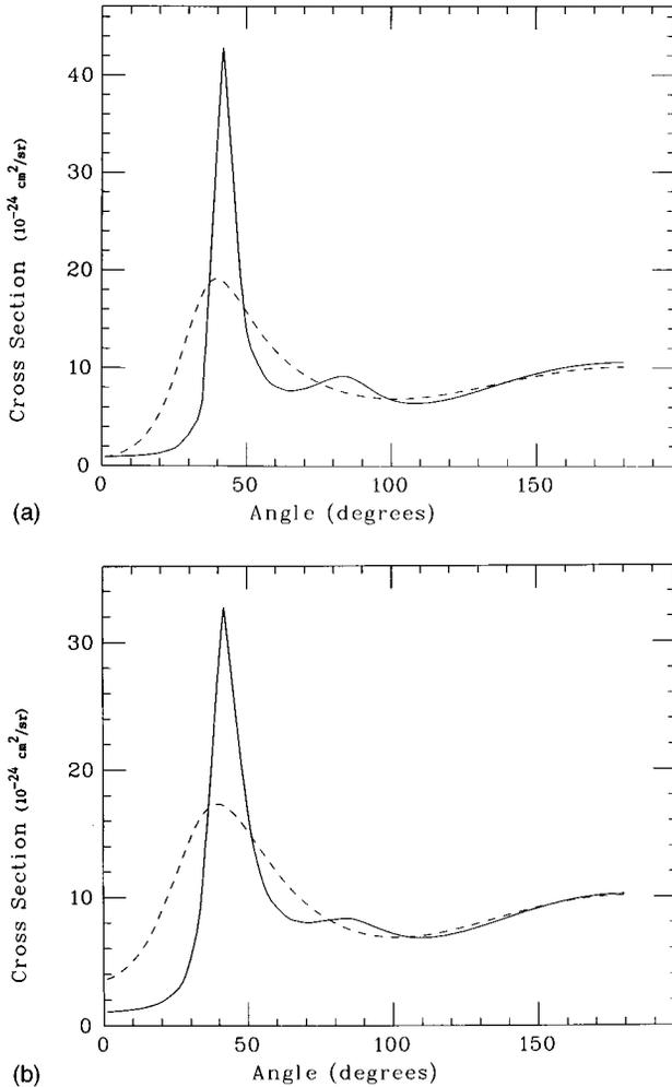
FIG. 3. Angular distribution of scattered x rays from Cu plasma that could be produced in a femtosecond laser plasma interaction experiment. The electron temperature is 100 eV. The ion temperatures are 100 eV for the dashed curve and 10 eV for the full curve. The plasma density is  $7.97 \text{ g/cm}^3$ , and the energy of the scattered x rays is 8 keV. (a) The calculation assumes no interionic screening. (b) The calculations assume interionic screening due to free electrons.
