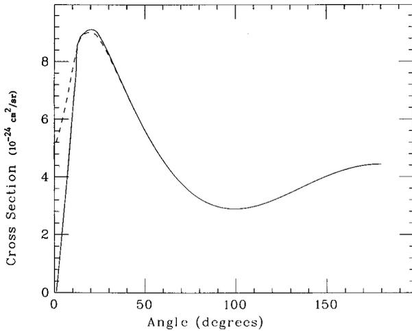
FIG. 1. Angular distribution of scattered x rays from an Al plasma of temperature 4 eV and density  $0.1 \text{ g/cm}^3$ . The energy of the scattered x rays is 4.75 keV. Full line: no screening of the ion-ion interaction. Dashed line: results of calculations assuming free-electron screening of the ion-ion interaction.
