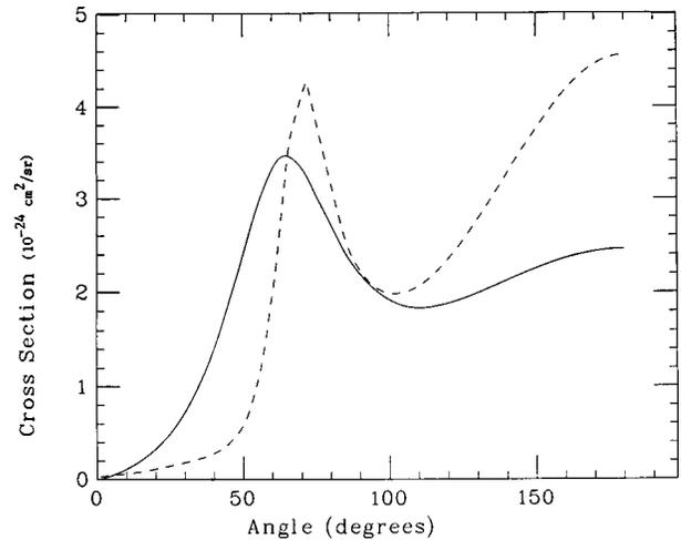
FIG. 2. Angular distribution of scattered x rays from an Al plasma of temperature 6 eV and density  $12 \text{ g/cm}^3$ . The energy of the scattered x rays is 7.47 keV. Full line: results using the procedure outlined in this paper. Dashed line: results using the Thomas-Fermi model as described in Ref. [3].
