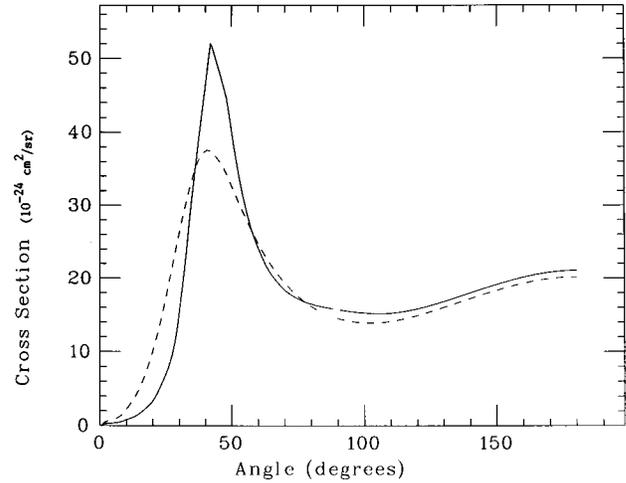
FIG. 4. Angular distribution of scattered x rays from Cu plasma that could be produced in a femtosecond laser plasma interaction experiment. The electron temperatures are 0.5 (full curve) and 5 eV (dashed curve). The ion temperatures in both cases are assumed to be equal to the electron temperature. The plasma density is  $8.93 \text{ g/cm}^3$ , and the energy of the scattered x rays is 8 keV. The calculations assume no interionic screening.
