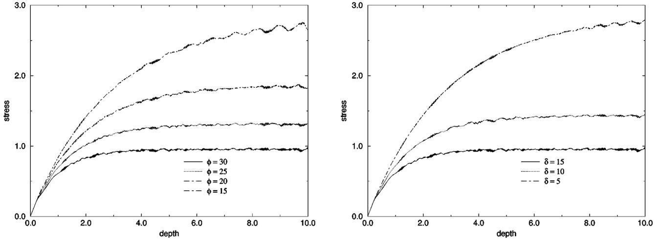
FIG. 4. (a) The  $yy$  component of the stress at the centerline for different nominal internal friction angles. The nominal wall friction is held fixed  $\delta=15^\circ$ . (b) The  $yy$  component of the stress at the centerline for different nominal wall friction angles, with a fixed nominal internal friction angle  $\phi=30^\circ$ .
