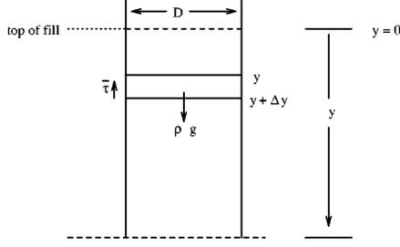
FIG. 1. Force balance for Janssen's analysis. On the slice, stresses and gravity are balanced by wall friction.
