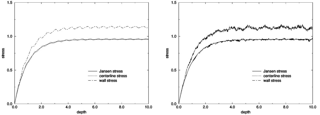
FIG. 2. (a) The  $yy$  component of the stress at the centerline and the wall, with no random component of friction. For comparison the Jansen solution is also plotted. Here the nominal internal friction angle  $\phi=30^\circ$  and the nominal wall friction angle  $\delta=15^\circ$ . (b) Similar plot, but with a random component added to the friction angles.
