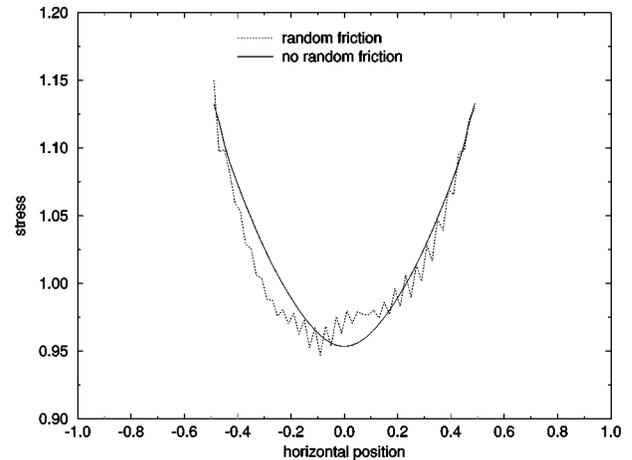
FIG. 3. Variation in the  $yy$  stress across the width of the bin, at  $y=10$ . Shown are results both with and without a random component of the friction angles. In both cases, the nominal friction angles are  $\phi=30^\circ$  and  $\delta=15^\circ$ .
