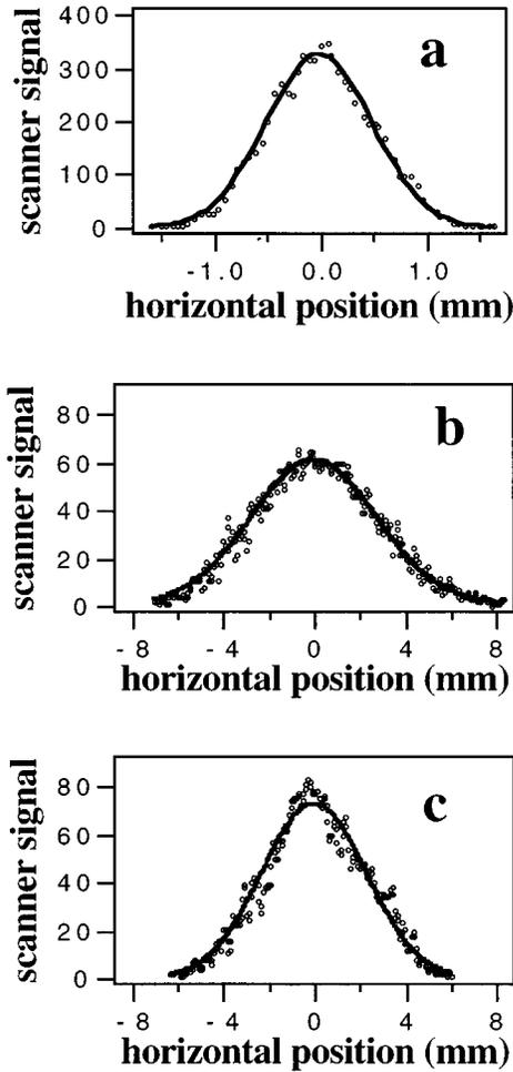
FIG. 2. Horizontal profile measured by the wire scanner at the spectrometer, where the scanner signal is proportional to the charge density and the circles are from measurement and the solid curves are Gaussian fittings. Profile (a) was measured with the zero-phasing cavities off while profiles (b) and (c) were measured with the zero-phasing cavities at  $+90^\circ$  and  $-90^\circ$  off the crest.
