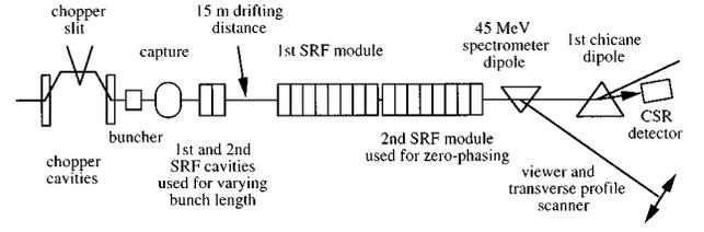
FIG. 1. Schematic block diagram of CEBAF injector layout.
