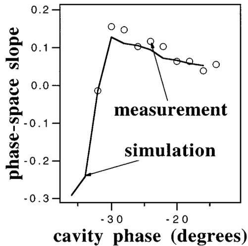
FIG. 4. The normalized longitudinal phase-space slopes. The circles are the measurement of the right-hand side of Eq. (8),  $(X_{\text{rms}}^+ - X_{\text{rms}}^-)/(X_{\text{rms}}^+ + X_{\text{rms}}^-)$ , while the solid curve is the left-hand side,  $(dE/dz)/(2\pi eV_{\text{rf}}/\lambda_{\text{rf}})$ , from simulation.
