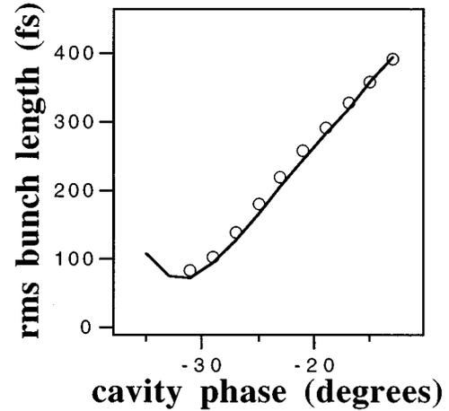
FIG. 3. The bunch length versus the second Srf cavity phase, where the circles are from measurement and the solid curve is from simulation.
