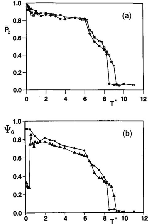
FIG. 4. Plots of order parameters as a function of scaled temperature for model I. The points are connected by lines to serve as a guide to the eye. (a) Second rank orientational order parameter  $\bar{P}_2$  ( $\square$ , heating;  $\bullet$ , cooling). (b) Bond order parameter  $\Psi_6$  ( $\triangle$ , heating;  $\bullet$ , cooling).
