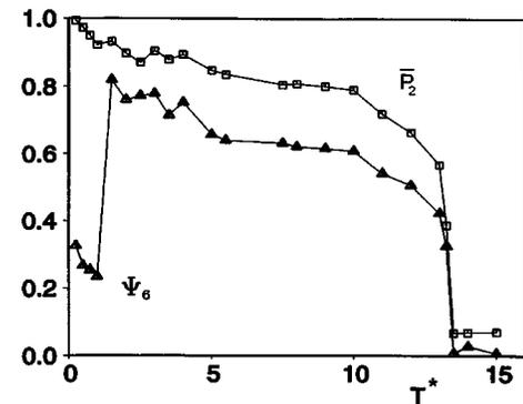
FIG. 10. Plots of the second rank orientational order parameter  $\bar{P}_2$  ( $\square$ ), and the bond order parameter  $\Psi_6$  ( $\triangle$ ) as a function of scaled temperature for model II.
