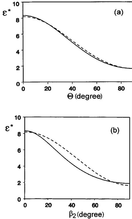
FIG. 2. Comparison of the scaled strength parameter  $\epsilon^* = \epsilon(\hat{u}_1, \hat{u}_2, \hat{r})/\epsilon_0$ , obtained from our model via Eq. (5) (dashed line), and GB via Eq. (6) (solid line). (a)  $\alpha_1 = \alpha_2 = \beta_1 = \beta_2 = \phi = 0^\circ$ , and  $\theta$  varied. (b)  $\alpha_1 = \alpha_2 = \phi = 0^\circ$ ,  $\beta_1 = \theta = 0^\circ$ , and  $\beta_2$  varied.
