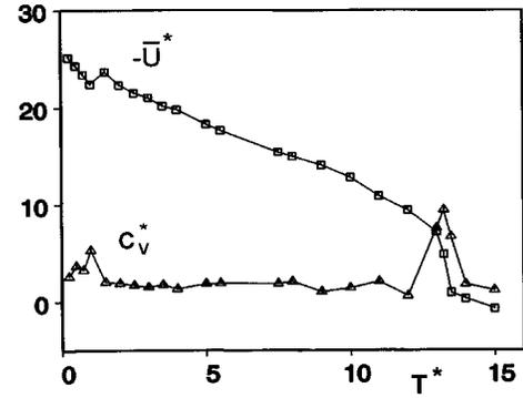
FIG. 9. The scaled internal energy  $\bar{U}^*(\equiv \langle U/N\epsilon_0 \rangle)$  ( $\square$ ) and heat capacity  $C_V^*(\equiv C_V/Nk)$  ( $\triangle$ ) as a function of scaled temperature  $T^*(\equiv kT/\epsilon_0)$  for model II.
