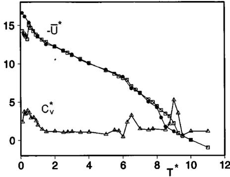
FIG. 3. The scaled internal energy  $\bar{U}^*(\equiv \langle U/N\epsilon_0 \rangle)$  ( $\square$ ) and heat capacity  $C_V^*(\equiv C_V/Nk)$  ( $\triangle$ ) as a function of the scaled temperature  $T^*(\equiv kT/\epsilon_0)$  for model I obtained from the heating run. The internal energy results obtained from the cooling run starting from the isotropic phase are indicated as ( $\bullet$ ). Lines are drawn through the points as a guide to the eye.
