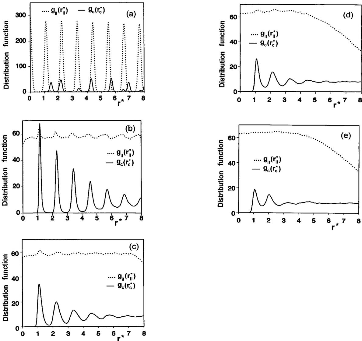
FIG. 8. Plots of pair distribution functions for model I:  $g_{\parallel}(r_{\parallel}^*)$  (dotted line) obtained via Eq. (9) and  $g_c(r_c^*)$  (solid line) obtained via Eq. (10) for five reduced temperatures. (a) 0.40 (fcc), (b) 0.5 ( $D_{ho}$ ), (c) 6.0 ( $D_{hd}$ ), (d) 8.0 ( $N_D$ ), (e) 10.0 (isotropic).
