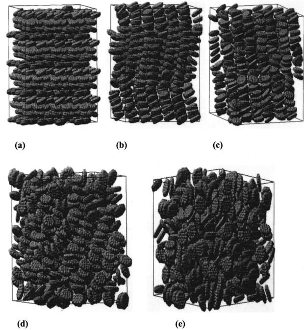
FIG. 5. Snapshots of final configurations for model I taken from the production stages at five reduced temperatures as viewed at an angle with respect to the director. For the sake of clarity the dimensions of the particles are scaled down by 20%. (a) 0.40 (fcc). (b) 0.5 ( $D_{ho}$ ). (c) 6.0 ( $D_{hd}$ ). (d) 8.0 ( $N_D$ ). (e) 10.00 (isotropic).
