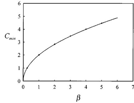
FIG. 3. The numerical calculations on the selected velocity  $C_{min}$  versus the parameter  $\beta$ . The solid line is the theoretical prediction by Eq. (19), and the filled circles represent the numerical results on Eq. (17).
