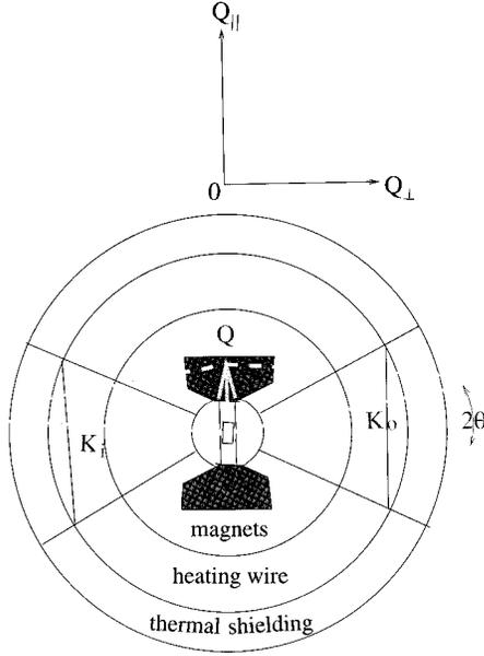
FIG. 2. The sample was mounted inside the oven and aligned with an *in situ* magnet field. The x-ray wave vectors  $K_i$  and  $K_o$  were defined by the incident beam and position of detector.  $2\theta$  is the scattering angle and  $\mathbf{Q}$  is the scattering vector.  $Q_{\parallel}$  is the component of  $\mathbf{Q}$  parallel to the long axis of the molecules defined by the magnetic field, and  $Q_{\perp}$  is the perpendicular component.
