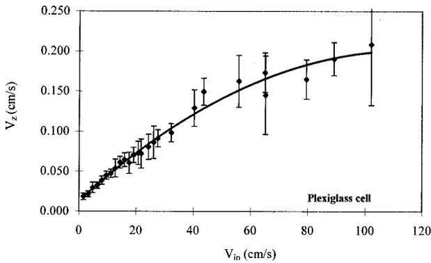
FIG. 7. Average vertical speed  $V_z$  of a 2 mm marker in a 1 mm glass medium vs inner cylinder speed in a plexiglass cell. The solid line represents a quadratic fit to the data.
