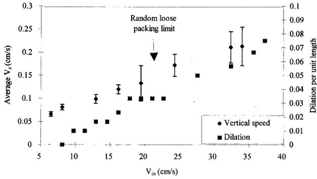
FIG. 4. Average vertical speed  $V_z$  of a 2 mm marker in a 1 mm medium and dilation per unit length of the medium vs the inner cylinder speed in a glass cell.
