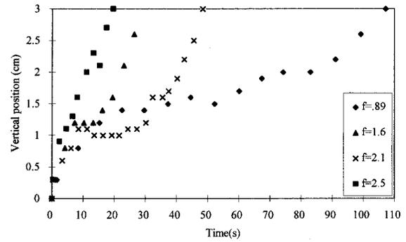
FIG. 2. Vertical position  $z$  of a 2 mm marker in a 1 mm medium vs time for various drive frequencies in a glass cell.
