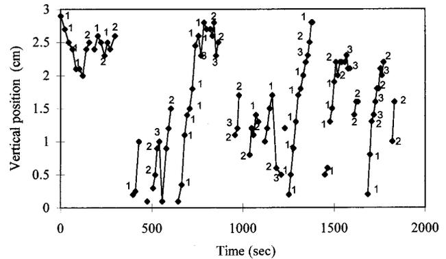
FIG. 6. Vertical position  $z$  of a 1 mm marker in a 1 mm medium vs time (glass cell). Inner cylinder speed is 8.95 cm/s. The absence of lines in some regions indicates that the marker was not visible on the monitor screen during those time intervals.
