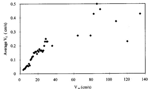
FIG. 3. Average vertical speed  $V_z$  of a 2 mm marker in a 1 mm medium vs speed of the inner cylinder in a glass cell.
