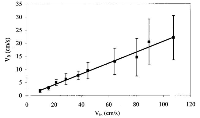
FIG. 5. Average horizontal speed  $V_\theta$  of the 2 mm marker in a 1 mm glass medium vs the inner cylinder speed (glass cell). The slope is  $\frac{1}{5}$ .
