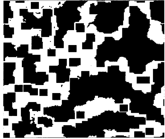
FIG. 4. The conducting pore space of the porous sample shown in Fig. 1 corresponding to an effective porosity \phi_{\text{eff}} = 0.40 .
