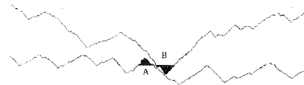
FIG. 2. Sketch for the definition of the energy released during an earthquake. It is assumed proportional to the breaking area [the (d-1) -dimensional sets A and B ] between the two asperities: E \propto A + B .
