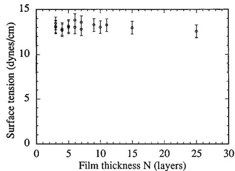
FIG. 3. Surface tension of H10F5MOPP as a function of film thickness which is essentially constant. The data were obtained during a thinning transition run.
