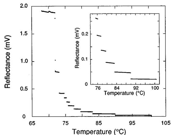
FIG. 1. Optical reflectance data showing thinning transitions in a free-standing film of H8F(4,2,1)MOPP. The original film thickness is about 25 layers. The inset highlights the negative slopes seen in all successive steps in the region of single-layer thinning ( $N \leq 7$ ) before the two-layer film ultimately ruptured above 100 °C.
