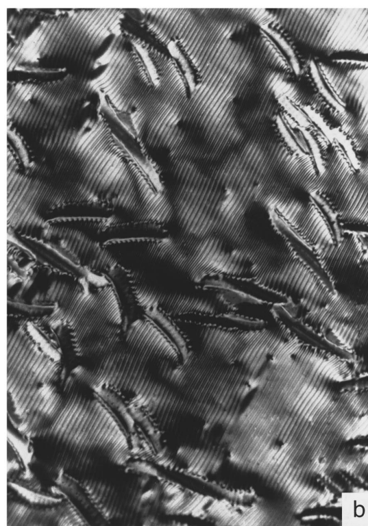
FIG. 2. (a) Two liquid-crystalline phases of DNA are shown in a sample of uniform concentration. The dark background is the cholesteric phase with twist axis perpendicular to the photograph. The brighter regions with extinction brushes are the columnar phase, growing slowly as an almost circular domain. (b) The same two phases at a uniform concentration, but aligned in a magnetic field of 6.4 T. The anisotropic growth of the narrow nonstriated columnar phase is seen clearly in contact with the cholesteric fingerprint texture.
