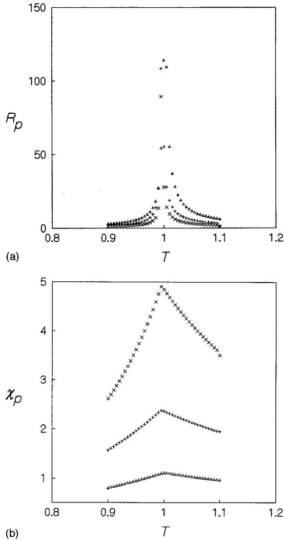
FIG. 5. Temperature variation of (a)  $R_p$  and (b)  $\chi_p$  for different values of  $\delta t$  in the mean-field case: the triangle is for  $\delta t = 8$ , the plus is for  $\delta t = 16$ , and the cross is for  $\delta t = 32$ .
