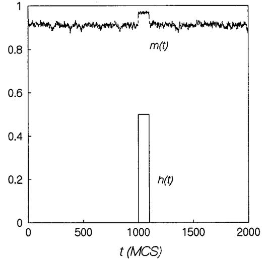
FIG. 1. Time variation of magnetic field  $h(t)$  and the response magnetization  $m(t)$  in the Monte Carlo case, for  $h_p = 0.5$  and  $\delta t = 50$ .
