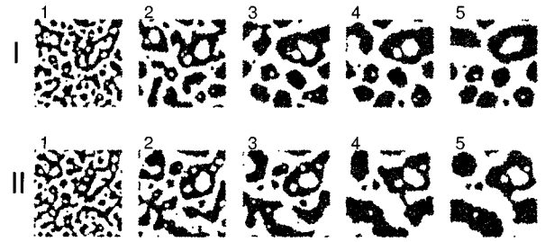
FIG. 6. Temporal evolution of phase-separating patterns by molecular dynamics at temperature k_B T = 0.04 ( \sqrt{k_B T} = 0.2 ). Two sequences labeled I and II start with slightly different initial conditions, namely, that the velocity of only one particle for sequence I is different from that for sequence II by an amount of only 10^{-10} . The number of particles is 64^2 .
