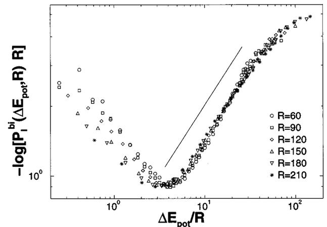
FIG. 3. Logarithm of the rescaled probability distribution of the dissipation of potential energy for the large disks in bidisperse systems. The width of the avalanche zone was  $w_{\text{az}}=0.15R$ . The slope of the solid line is the mean value of the exponent  $\gamma_{\text{bi}}$  for all system sizes and avalanche zone widths.
