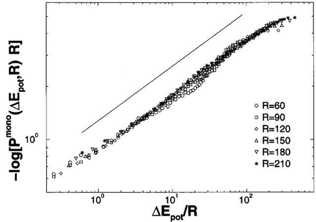
FIG. 4. Logarithm of the rescaled probability distribution of the dissipation of potential energy for monodisperse systems. The width of the avalanche zone was  $w_{\text{az}} = 0.15R$ . The slope of the solid line is the mean value of the exponent  $\gamma_{\text{mono}}$  for all system sizes and avalanche zone widths.
