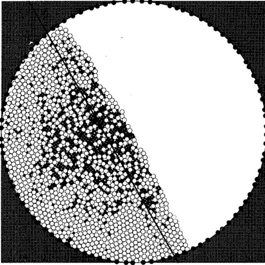
FIG. 1. A drum of radius  $R=60$  after three total revolutions of the drum with small black and large white disks. The large black disks on the wall of the drum are randomly spaced fixed ones in order to increase the disorder in the structure of the filling. The solid line at a distance  $0.2R$  from the center of the drum indicates the avalanche zone. Its angle to the horizontal is the averaged angle of repose  $\alpha_r=60.44^\circ$  in this system.
