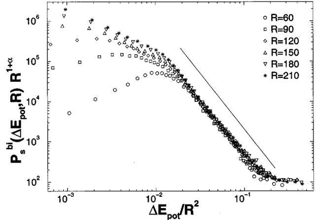
FIG. 2. Rescaled probability distribution of the dissipation of potential energy for the small disks in bidisperse systems. The width of the avalanche zone was  $w_{\text{az}}=0.15R$ . The solid line indicates the obtained slope of the power law area  $\alpha=2.8$  for all system sizes and avalanche zone widths.
