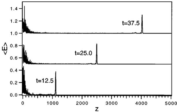
FIG. 2. Average kinetic energy as a function of depth for sound propagation in two-dimensional column with 3.3% void fraction,  $v_{\text{impact}}=0.1$ , and  $n=5/2$ .
