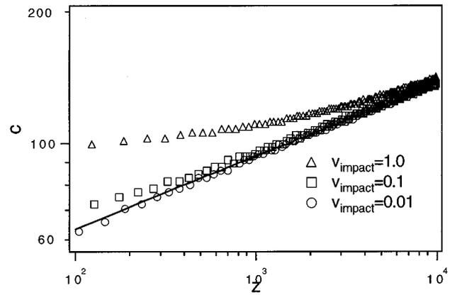
FIG. 3. Speed of vertical disturbances as a function of depth,  $c$  vs  $z$ , with the solid line showing the scaling law predicted by Hertzian contact theory. The calculations have been done for  $n=5/2$  in one dimension. The slope is  $1/6$ .
