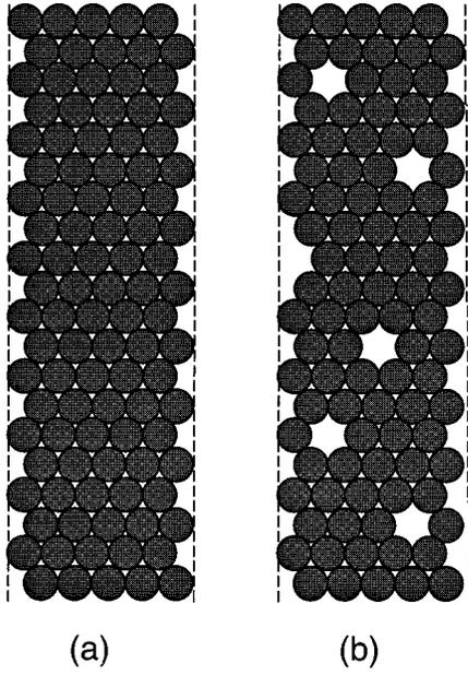
FIG. 1. (a) A pristine two-dimensional granular column. (b) A column with randomly distributed voids as discussed in Sec. II C.
