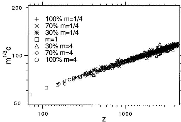
FIG. 11. Mass-scaled speeds of vertical disturbances in granular columns with mass defects for  $n=5/2$  in the limit of weak perturbations. Legend refers to the fraction of  $m=1$  grains that have been replaced by mass defects.
