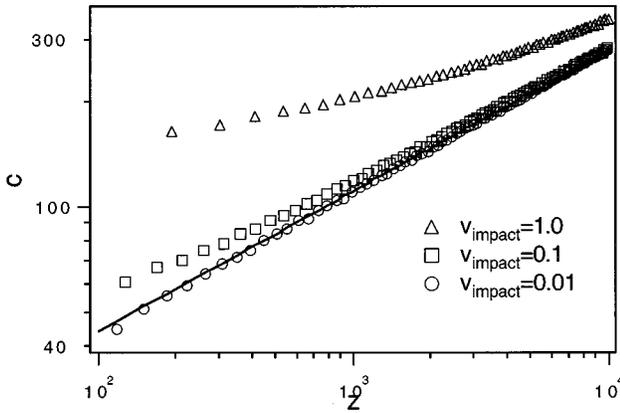
FIG. 4. Plot of  $c$  vs  $z$  for  $n=6$  in one dimension. The slope of the solid line predicted by Hertzian contact theory is  $2/5$ .
