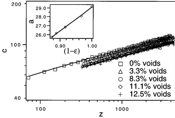
FIG. 9. Speed of the vertical disturbance in two-dimensional columns with voids for  $n=5/2$  in the limit of weak impact. Solid lines are the best fits to data of form  $c=az^b$ . Inset shows the prefactor  $a$  plotted against  $1-\epsilon$ . The linear behavior of  $a$  for small  $\epsilon$  suggests that  $c \propto (1-\epsilon)z^{1/6}$ .
