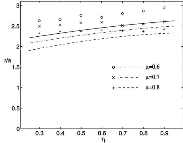
FIG. 8. Ratio of halo radius to the matched beam radius vs tune depression  $\eta$  for mismatch  $\mu=0.6, 0.7, 0.8$ . Curves show predictions of the analytical model.
