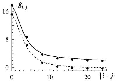
FIG. 5. Spatial correlation function  $g_{ij}$ , Eq. (12), as a function of  $|i-j|$  for the model (16). The solid and the dashed curves correspond to the numerical solution of the master equation for  $\delta=3 \times 10^{-3}$  and  $\delta=10^{-2}$ , respectively. The circles are obtained through the corresponding microscopic simulation based on Bird's algorithm. The statistics is taken over enlarged cells of about 4 mean free paths long. The parameters are given in Eq. (25).
