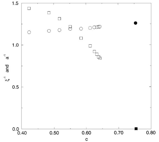
FIG. 2. Parameters of the fit of  $g(r)$  to Eq. (3),  $\xi^{-1}$  (squares) and  $a^{-1}$  (circles), as a function of  $c$ . The filled symbols indicate their expected extrapolations for  $c=c_0$  (see the text).
