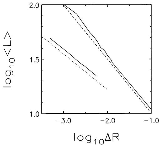
FIG. 6. Same as in Fig. 3, but now for a square  $200 \times 200$  plate with the PD Eq. (4) with  $f_{\min}=100$  and  $W=10$  (upper curve) and with the PD Eq. (5) with  $W=100$  (lower curve). Note the double-logarithmic scales. Again, the dashed line has a slope  $-\frac{1}{2}$ , the dotted line a slope  $-\frac{1}{3}$ .
