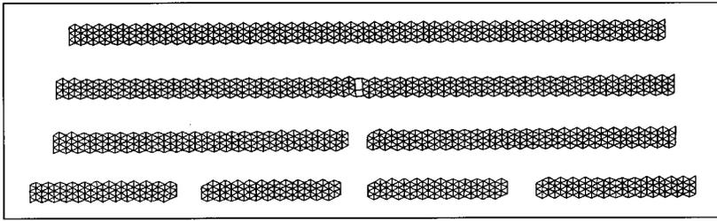
FIG. 2. Series of fragmentation stages of an elongated strip under uniaxial stress.
