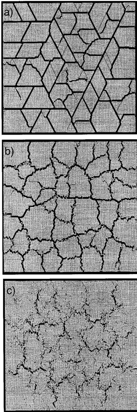
FIG. 4. Fragmentation patterns on a  $150 \times 150$  lattice with  $\xi=20$  after 4000 bonds have failed; the PD is Eq. (4), with  $f_{\min}=100$ . Furthermore,  $W$  is 15 in (a), 100 in (b), and 400 in (c).
