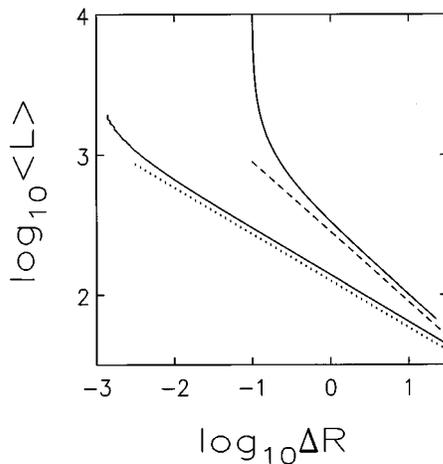
FIG. 3. Mean fragment size  $L$  as a function of  $\Delta R$  (the elongation of the substrate) in a quasi-1D geometry (a  $50 \times 25000$  strip) plotted in double-logarithmic scales. The upper curve corresponds to the PD Eq. (4), with  $f_{\min}=100$  and  $W=10$ , the lower curve to the PD Eq. (5) with  $W=100$ . The numerical results were obtained using an average over ten realizations each. The slope of the dashed line is  $-\frac{1}{2}$  and that of the dotted line is  $-\frac{1}{3}$ .
