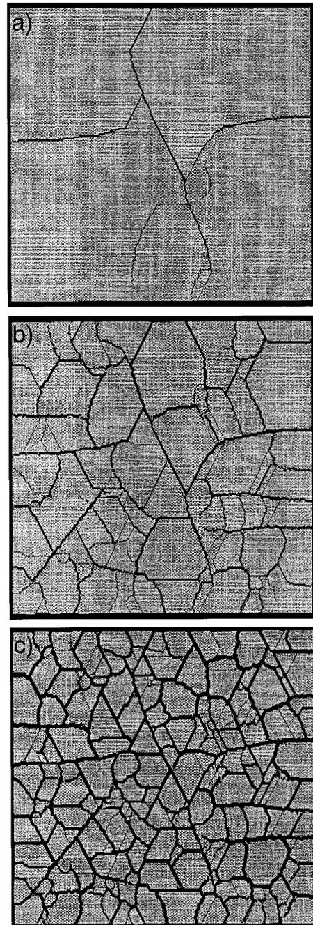
FIG. 5. Fragmentation patterns on a  $200 \times 200$  lattice with  $\xi=150$  after 1000, 5000, and 10 000 bonds have failed. The PD is Eq. (4) with  $f_{\min}=200$  and  $W=10$ .
