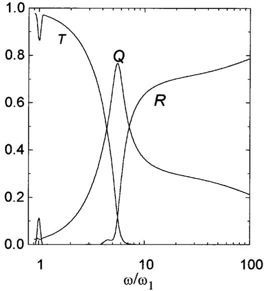
FIG. 7. Frequency dependence of the coefficients of reflection, transmission, and absorption of radiation incident upon the AIR at an angle of  $\theta_i=30^\circ$ .
