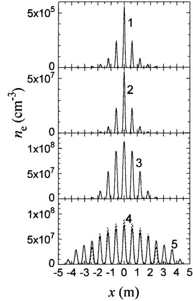
FIG. 5. Profiles of electron concentration in the AIR after passage of  $n$  microwave pulses ( $n_1=25$ ,  $n_2=35$ ,  $n_3=45$ ,  $n_4=70$ ,  $n_5=200$ ). The discharge parameters:  $\omega=\pi \times 10^9$  s $^{-1}$ ,  $2E_a=143$  V/cm,  $\tau_0=25$  ns,  $F^{-1}=7.2$  ms,  $h=55$  km,  $R_0=200$  m,  $\theta=60^\circ$ .
