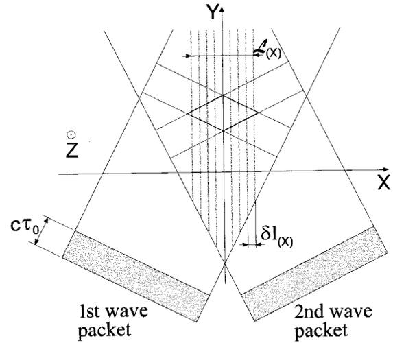
FIG. 1. The AIR structure in the case of short maintaining microwave pulses.
