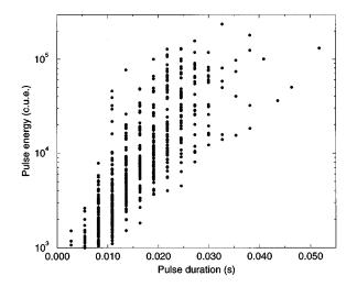
FIG. 1. Scatter plot of pulse duration versus pulse energy for cylindrical weak crumpling of Xerox 4024 paper with a 2-in. triangular grid. Horizontal axis is linear, vertical axis is logarithmic. Energy is measured in units of computer unit amplitude squared over time in seconds (computer unit energy or c.u.e.).
