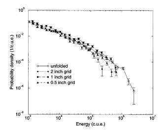
FIG. 7. Weak crumpling of triangularly gridded Xerox 4024 paper, normalized to 50 cycles. No systematic dependence of pulse energy distribution on grid scale is seen.
