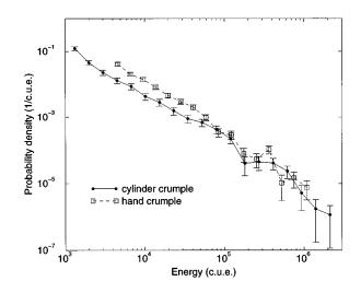
FIG. 4. Strong cylindrical crumples and hand crumples: Xerox 4024 duplicator paper was crumpled strongly in hand and using the cylindrical method. In both cases a sum of three crumpling runs is shown. Error bars are  $\pm 1 \sigma$  predicted by Poisson statistics.
