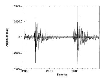
FIG. 3. Sound amplitude versus time: two adjacent pulses identified by our algorithm. The spacing of minor ticks is equal to the time bin duration in which energy was integrated, and the two superimposed lines show the threshold value. Bins were considered "active" when the energy inside equaled the bin length times the threshold amplitude squared.
