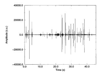
FIG. 2. Sound amplitude versus time: one entire strong cylindrical crumple, Xerox 4024 paper 8.5 in. square. Amplitude is measured in computer units (c.u.), signed 16-bit integers used to represent sound amplitude in digital recording.
