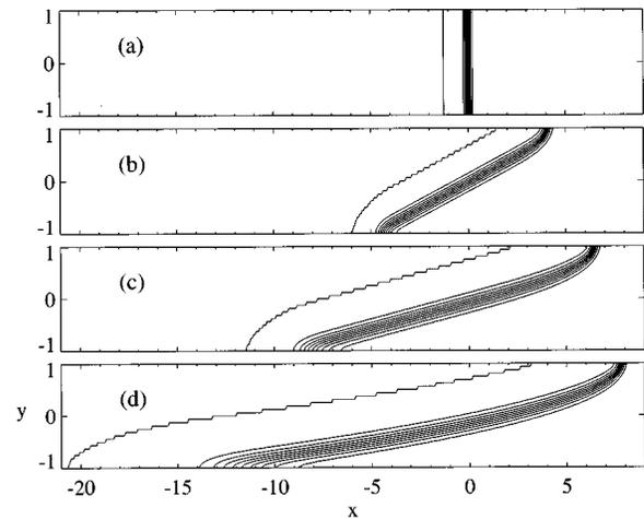
FIG. 2. Contour plots of  $b$  showing the evolution of a plane-wave front in the presence of the linear shear flow  $U=100y$  at times  $t_a=0$ ,  $t_b=0.05$ ,  $t_c=0.1$ , and  $t_d=1$ . The region containing  $B$  only is on the left-hand side, and for this and subsequent figures, the contour levels are at intervals of 0.1.
