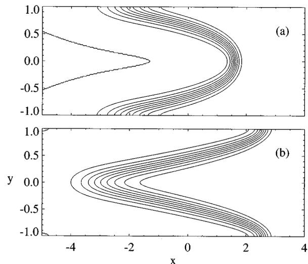
FIG. 3. Final forms of the wave fronts in the presence of the parabolic shear flows: (a)  $U=100(1-y^2)$  and (b)  $U=-100(1-y^2)$ .
