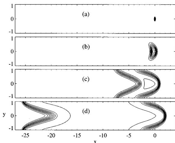
FIG. 4. Evolution of the initial condition  $b = \exp[-100(x^2 + y^2)]$  subjected to the parabolic shear flow  $U = -100y^2$ .  $t_a = 0$ ,  $t_b = 0.1$ ,  $t_c = 0.2$ , and  $t_d = 0.4$ .
