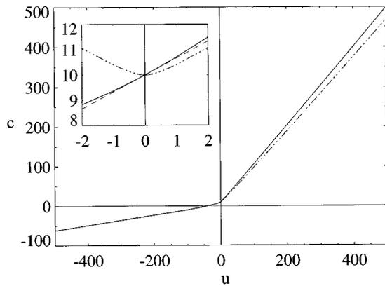
FIG. 1. Shear amplitude-wave-front velocity plot. The full curve is for parabolic shear; the dash-dotted curve is for linear shear. The inset shows the behavior for small-amplitude shears. The broken line is the first-order result from the perturbation analysis for a parabolic shear. The wave-front velocity for a linear shear is an even function of  $u$ . For clarity, the positive  $u$  results reflected about  $u=0$  are shown only in the inset.
