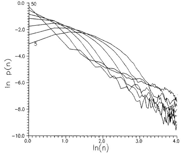
FIG. 4. The transient to a power function of the probability distribution  $P(n)$  of laminar phase size  $n$ , where  $n$  is the number of integral steps throughout the laminar phase. The sampling interval  $T$  is of the different values  $5\Delta t, 7\Delta t, 10\Delta t, 15\Delta t, 20\Delta t, 30\Delta t$ , or  $50\Delta t$ , respectively. Here,  $\Delta t$  is the integral step of time  $t$ . The values of the parameters are the same as in Fig. 1.
