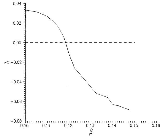
FIG. 2. The largest Lyapunov exponent of response subsystem with  $\alpha=0.1$ ,  $A=10.0$ ,  $\omega=1.0$ , and  $\beta=0.10-0.15$ .
