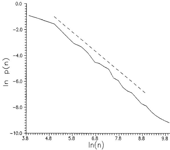
FIG. 5. The distribution of laminar phase size. The symbols  $P(n)$  and  $n$  are of the same meaning as Fig. 4. The sampling interval  $T$  is  $10\Delta t$ . The dashed line of slope  $-3/2$  is plotted to guide the eyes. A coarse grain technique is used to get this result that the occurrence probability of length from  $100n\Delta t$  to  $100(n+1)\Delta t$  is summed up and regarded as probability of length  $100(n+1/2)\Delta t$ .
