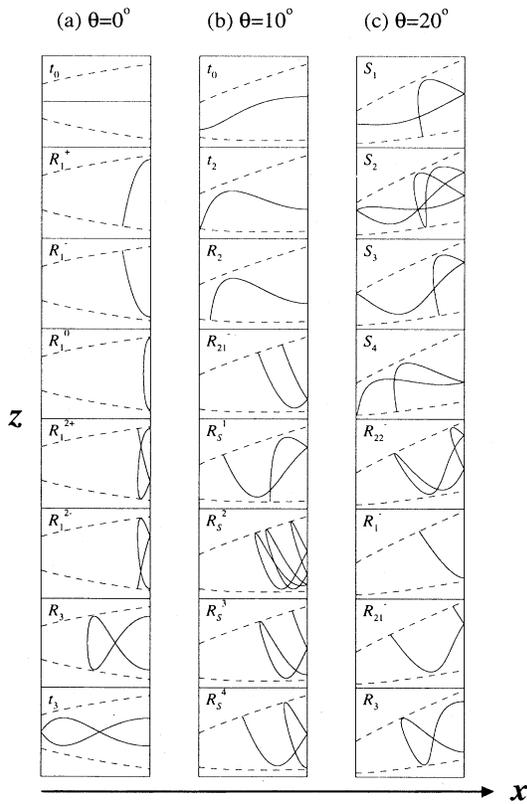
FIG. 4. Shapes of classical periodic orbits at (a)  $\theta = 0^\circ$ , (b)  $\theta = 10^\circ$ , and (c)  $\theta = 20^\circ$ . The broken lines indicate turning surfaces. The  $x$  axis spans the quantum well width from  $x = 0$  to  $x = L = 1200 \text{ \AA}$ . The vertical axis represents  $z$  in the same units.
