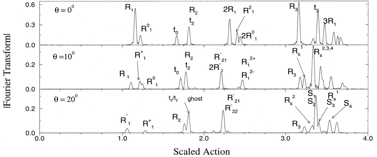
FIG. 3. Fourier transforms of the energy-level spectrum at  $\epsilon = 1.75 \times 10^3$  and  $\mathcal{E} = 600\epsilon$  for (a)  $\theta = 0^\circ$ , (b)  $\theta = 10^\circ$ , and (c)  $\theta = 20^\circ$ . Contributions from the most important periodic orbits have been identified. The same units as in Fig. 2 are used.
