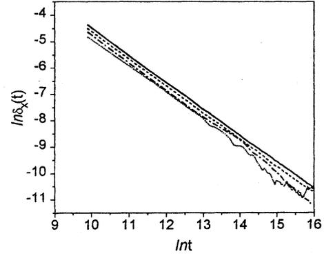
FIG. 10. The log-log (with base  $e=2.718\ 281\ 83\dots$ ) histogram of  $\delta_x(t)$  vs  $t$  in the two-dimensional motion case for the different radius of balls:  $r=5$  (dot-dashed), 10 (dashed), 15 (solid), 20 (dotted). Long straight segments indicates the power-law decay of  $\delta_x(t)$ .
