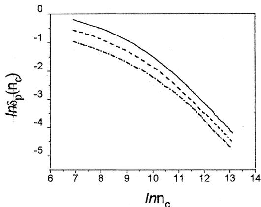
FIG. 6. The log-log (with the base  $e=2.718\ 281\ 83\dots$ ) histogram of  $\delta_p(n_c)$  vs  $n_c$  in the two-dimensional motion case for the different number of balls:  $N=2$  (dot-dashed), 6 (dashed), 12 (solid). Long straight segments exist in the long time limit, indicating the power-law decay of  $\delta_p(n_c)$ .
