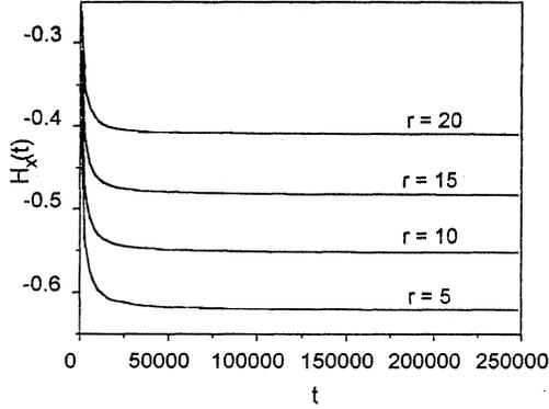
FIG. 9. The evolution of the Boltzmann's entropy  $H_x(t)$  for the 2D and two-ball case for the different radius of the balls. From upper to lower we take  $r=5, 10, 15, 20$ , respectively. It is shown that  $H_x(t)$  decreases monotonically and approaches its equilibrium value as time goes to infinity.
