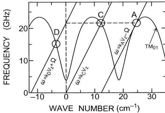
FIG. 4. The dispersion characteristics of the slow-wave ECM at the axial magnetic field of 0.76 T for the beam energy of 35 keV.
