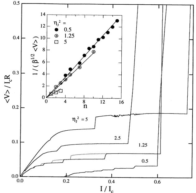
FIG. 2. Calculated  $IV$  curves for  $f = 1/8$ ,  $\beta = 61$ , and several values of the anisotropy parameter  $\eta_J$ . The inset shows the voltages of steps corresponding to locking number  $n$  determined from our numerical result compared to those calculated from Eq. (4) (solid lines).
