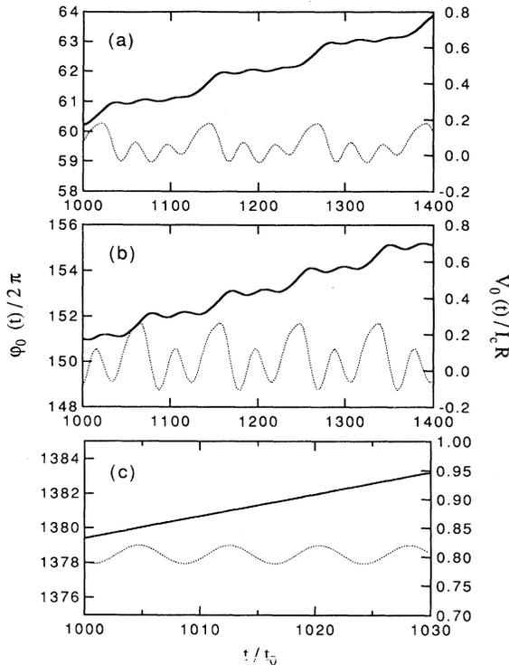
FIG. 3. Local phase difference  $\varphi_i(t)$  (solid lines) and voltage  $V_i(t)$  (broken lines) for  $i = 0$ ,  $f = 1/8$ ,  $\eta_J^2 = 1.25$ ,  $\beta = 61$ , and three values of the applied current:  $I/I_c = 0.22$  and  $0.41$ , corresponding to currents on voltage plateaus with  $n = 3, 2$ ; and  $I/I_c = 0.8$ , corresponding to a current in the whirling regime. Note the different scales in the axes for the whirling regime.
