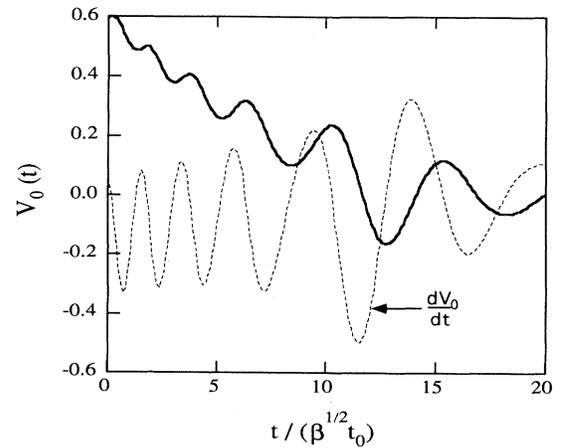
FIG. 4. Plot of  $V_0(t)$  and  $dV_0(t)/dt$  at  $x = 0$  after driving current is turned off at time  $t = 0$ . We use  $\eta_J^2 = 5$ , and  $I/I_c = 0.41$ , corresponding to an  $n = 1$  voltage plateau.
