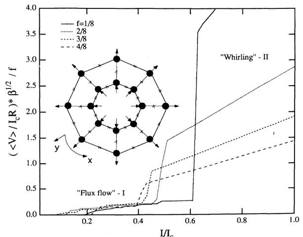
FIG. 1. Calculated  $IV$  curves for various values of  $f$  in an  $8 \times 1$  ladder ring.  $f \equiv Ba^2/\phi_0 = 1/8$  is the number of flux quanta per plaquette. We use  $\beta = 33$  and  $\eta_J = 0.71$ . Plotted voltages are divided by  $f$ . Inset: schematic of ring topology used in simulation. A uniform current is injected into the inner grains and drawn out from the outer grains.
