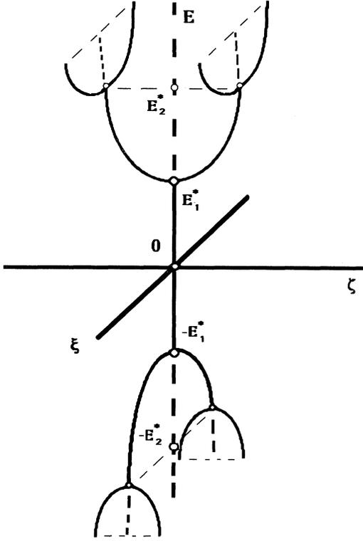
FIG. 5. Bifurcation tree of the Fréedericksz transition in tetrahedral nematic ( $\mathbf{E} \parallel \bar{C}_4$ ):  $\pm E_1^*$  and  $\pm E_2^*$  are the primary and the secondary bifurcation points, respectively.
