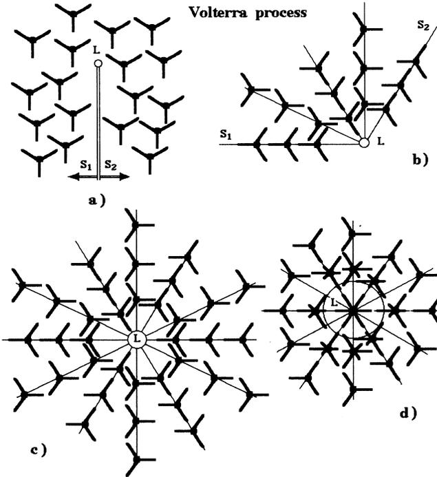
FIG. 7. The origin of the disclination line in the tetrahedral nematic via the Volterra process. Disclination line  $L$  is along the threefold rotational axis  $C_{3v}$  (normal to the plane of the page): (a) the cross section of the tetrahedral nematic LC by the plane  $L-S_1S_2$ ; (b) the displacement of the lips  $L-S_1$  and  $L-S_2$  of the cutting surface with respect to each other; (c) the disclination line  $L$  after viscous relaxation of the structure; (d) disclination core.
