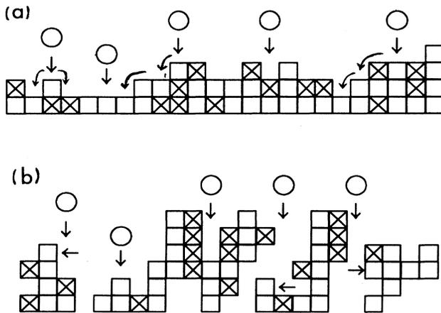
FIG. 1. Two deposition models: (a) The randomlike deposition model; (b) the ballisticlike deposition model. The circles represent the falling particles (particle  $A$  or particle  $C$ ), the squares represent particle  $A$ 's, and the squares with a cross denote particle  $C$ 's. The down arrows show the falling and the right and left arrows show the positions where the falling particle will stick.
