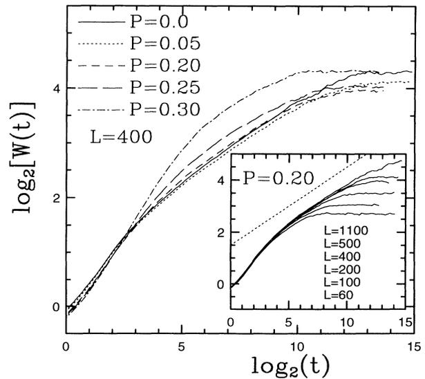
FIG. 6.  $\log_2 W(t)$  versus  $\log_2 t$  for the ballisticlike deposition model with all the parameters shown in the figure. The slope of the dashed line (in the inset) gives  $\beta = 0.30 \pm 0.01$ .
