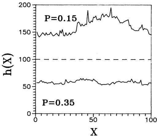
FIG. 5. Surface structure in the steady state of the randomlike deposition model for the system size  $L = 100$ : curve (a) for  $P = 0.15$  and curve (b) for  $P = 0.35$ . Only the region close to the surface is shown.
