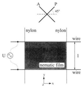
FIG. 2. A schematic diagram showing the experimental setup as viewed from above. The film is spread between two molybdenum wires spaced a distance  $\ell$  apart. A voltage  $U$  is applied between the wires to lift the azimuthal degeneracy of the director orientation in the plane of the film.
