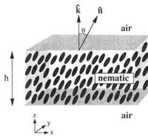
FIG. 1. A schematic diagram showing the orientation of the nematic director ( $\hat{\mathbf{n}}$ ) with respect to the surface normal ( $\hat{\mathbf{k}}$ ) of a freely suspended film. The film is bounded on both sides by air and has a thickness  $h$ .
