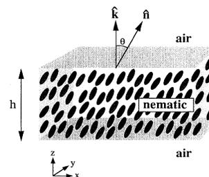
FIG. 1. A schematic diagram showing the orientation of the nematic director ( $\hat{\mathbf{n}}$ ) with respect to the surface normal ( $\hat{\mathbf{k}}$ ) of a freely suspended film. The film is bounded on both sides by air and has a thickness  $h$ .
