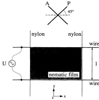
FIG. 2. A schematic diagram showing the experimental setup as viewed from above. The film is spread between two molybdenum wires spaced a distance  $l$  apart. A voltage  $U$  is applied between the wires to lift the azimuthal degeneracy of the director orientation in the plane of the film.
