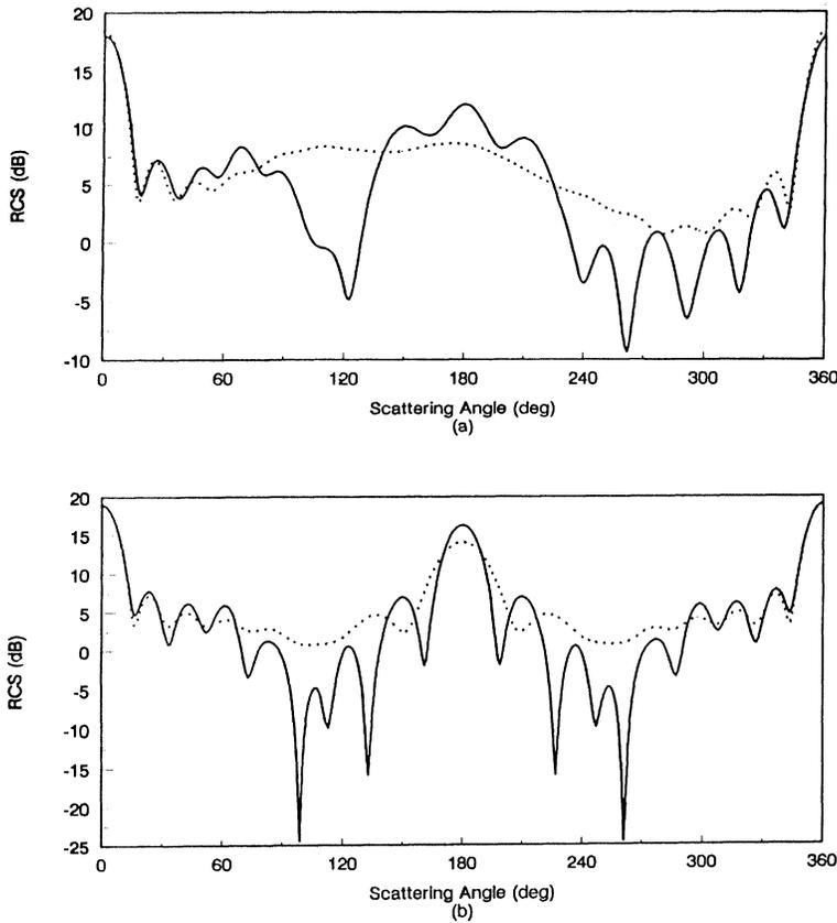
FIG. 6.  $E$  polarization, bistatic RCS  $\sigma/\lambda$  (dB),  $\varphi^{\text{inc}}=180^\circ$ ,  $kb=10$ ,  $ka=5$  (solid line), and  $ka=7.5$  (dotted line). (a)  $\mu_{xx}=1.5\mu_0$ ,  $\mu_{yy}=2.5\mu_0$ ,  $\mu_{xy}=-\mu_{yx}=3\mu_0$ , and  $\epsilon_{zz}=1.5\epsilon_0$ . (b)  $\mu_{xx}=\mu_0$ ,  $\mu_{yy}=4\mu_0$ ,  $\mu_{xy}=\mu_{yx}=0$ , and  $\epsilon_{zz}=2\epsilon_0$ .
