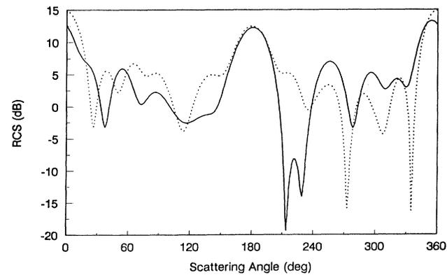
FIG. 7.  $E$  polarization, bistatic RCS  $\sigma/\lambda$  (dB),  $\varphi^{\text{inc}}=180^\circ$ ,  $a=0.5b$ ,  $kb=6$  (solid line),  $kb=8$  (dotted line),  $\mu_{xx}=1.5\mu_0$ ,  $\mu_{yy}=2.5\mu_0$ ,  $\mu_{xy}=-\mu_{yx}=3\mu_0$ , and  $\epsilon_{zz}=1.5\epsilon_0$ .
