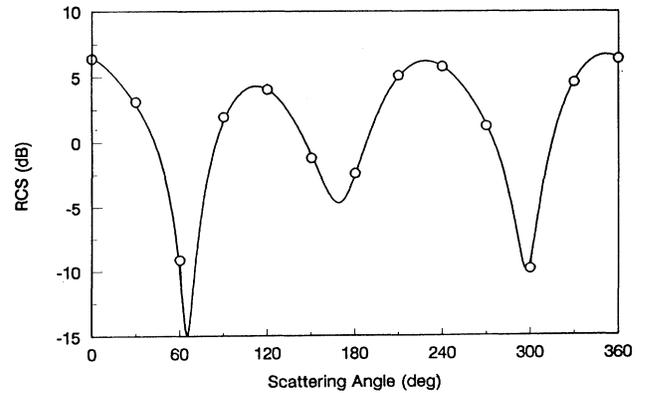
FIG. 5.  $E$  polarization, bistatic RCS  $\sigma/\lambda$  (dB),  $\varphi^{\text{inc}}=180^\circ$ ,  $\mu_{xx}=1.5\mu_0$ ,  $\mu_{yy}=2.5\mu_0$ ,  $\mu_{xy}=-\mu_{yx}=3\mu_0$ ,  $\epsilon_{zz}=1.5\epsilon_0$ ,  $ka=1$ , and  $kb=2$ . The markers are the solution taken from Ref. [9] [Fig. 6(c)].
