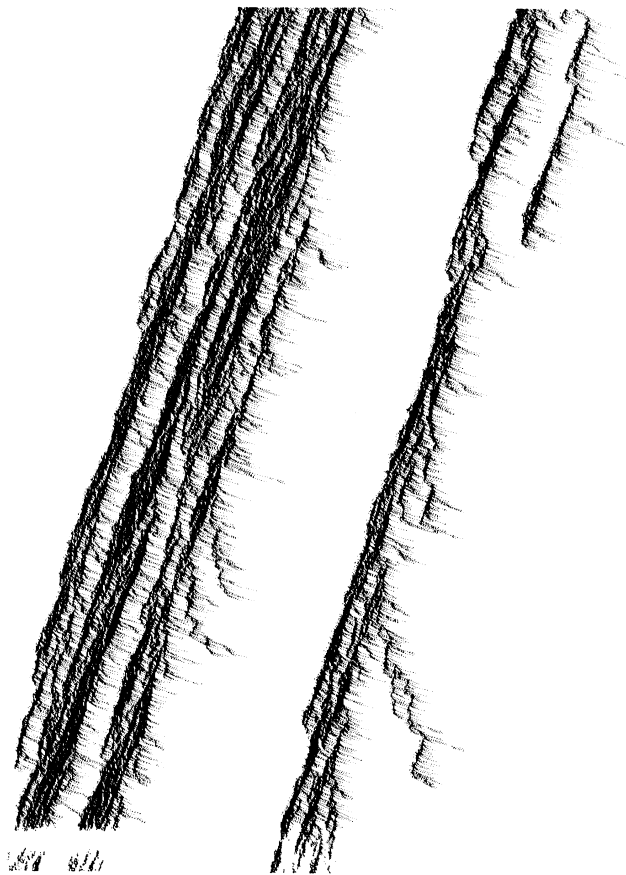
FIG. 3. Space-time plot of an emergent jam. The horizontal direction is space and the vehicle direction is time, as in Fig. 2. Only vehicles with v < v_{\text{max}} , i.e., “particles,” are plotted.
