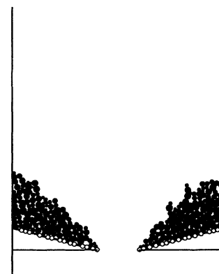
FIG. 4. Due to static friction, 314 particles remain in the hopper for an opening angle of \theta=150^\circ ( \gamma=100 Hz, \gamma_s=0 Hz, k_s=1000 g/s 2 , D=10d_0 , and \mu=0.5 ).
