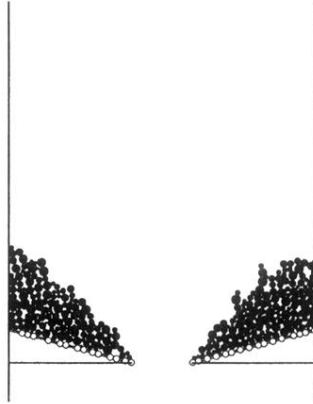
FIG. 4. Due to static friction, 314 particles remain in the hopper for an opening angle of \theta=150^\circ ( \gamma=100 Hz, \gamma_s=0 Hz, k_s=1000 g/s 2 , D=10d_0 , and \mu=0.5 ).
