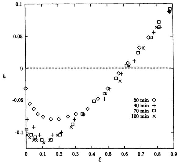
FIG. 2. Complete surface shapes measured at a constant rotation rate,  $\Omega=1.22$  using measurement method (i) as described in the text. Note the continuing evolution of the surface. The error in each measurement is on the order of the symbol size.
