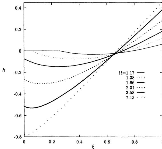
FIG. 1. Predicted surface shape  $h(\xi)$  as a function of rotation frequency for a system beginning with a flat upper surface and  $\theta_f = 34.6$ . Note the nondeforming central region at the lowest rotation rates. At intermediate values of  $\Omega$ , this leads to a cusp at  $\xi = 0$  which flattens out at higher  $\Omega$ . At these highest rotation frequencies, the slope becomes nearly constant at large  $\xi$ .
